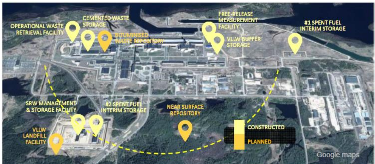
Figure 10. Ignalina NPP New Waste Facilities
