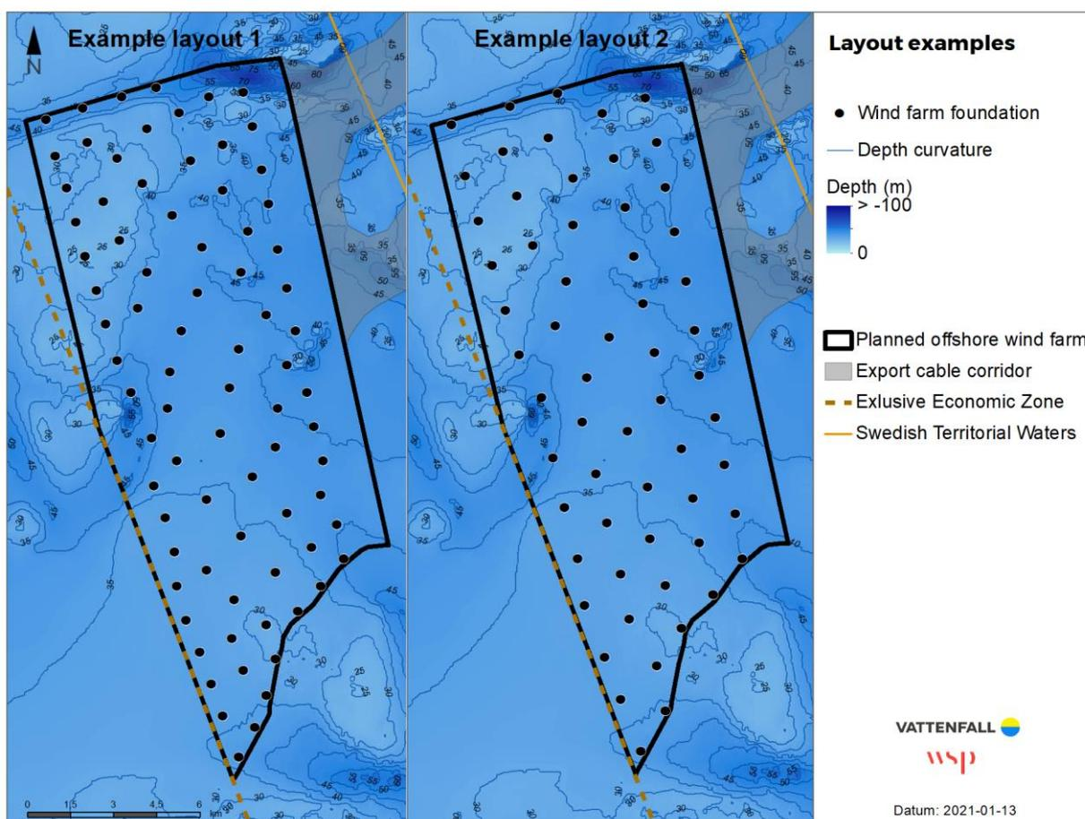
Figure 4. Two different examples of wind farm layouts. Example 1 illustrates 80 turbines with a total height of 260 m. Example 2 illustrates 60 turbines with a total height of 350 m (data source: depth from EMODnet).
