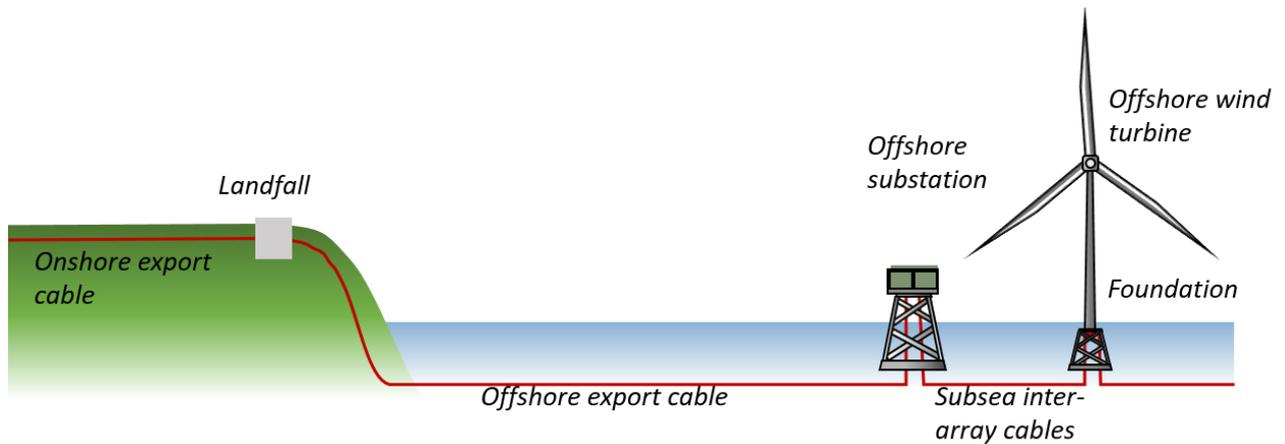
Figure 3. Schematic of an offshore wind farm, including all its parts.
