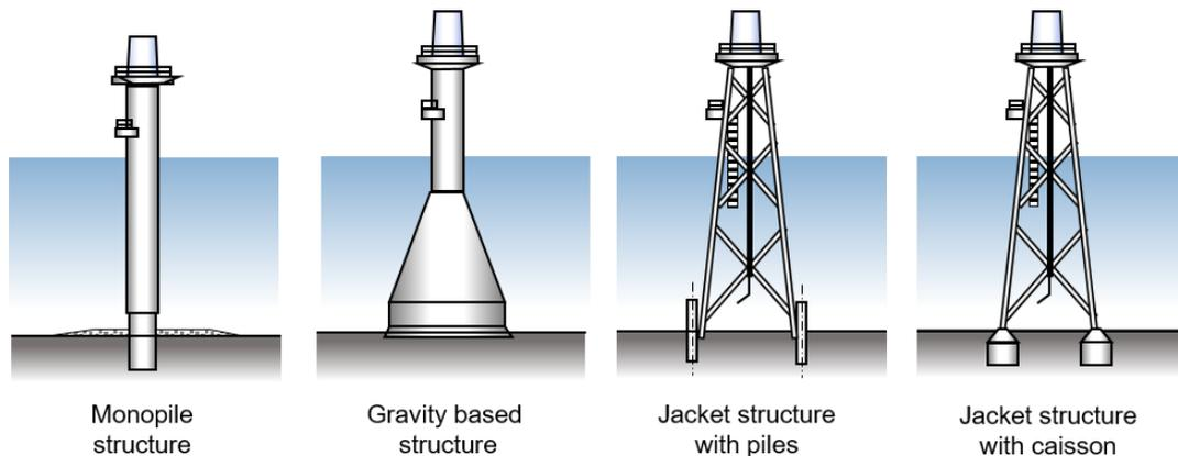
Figure 6. The different types of foundations currently applicable in Kattegatt Syd.
