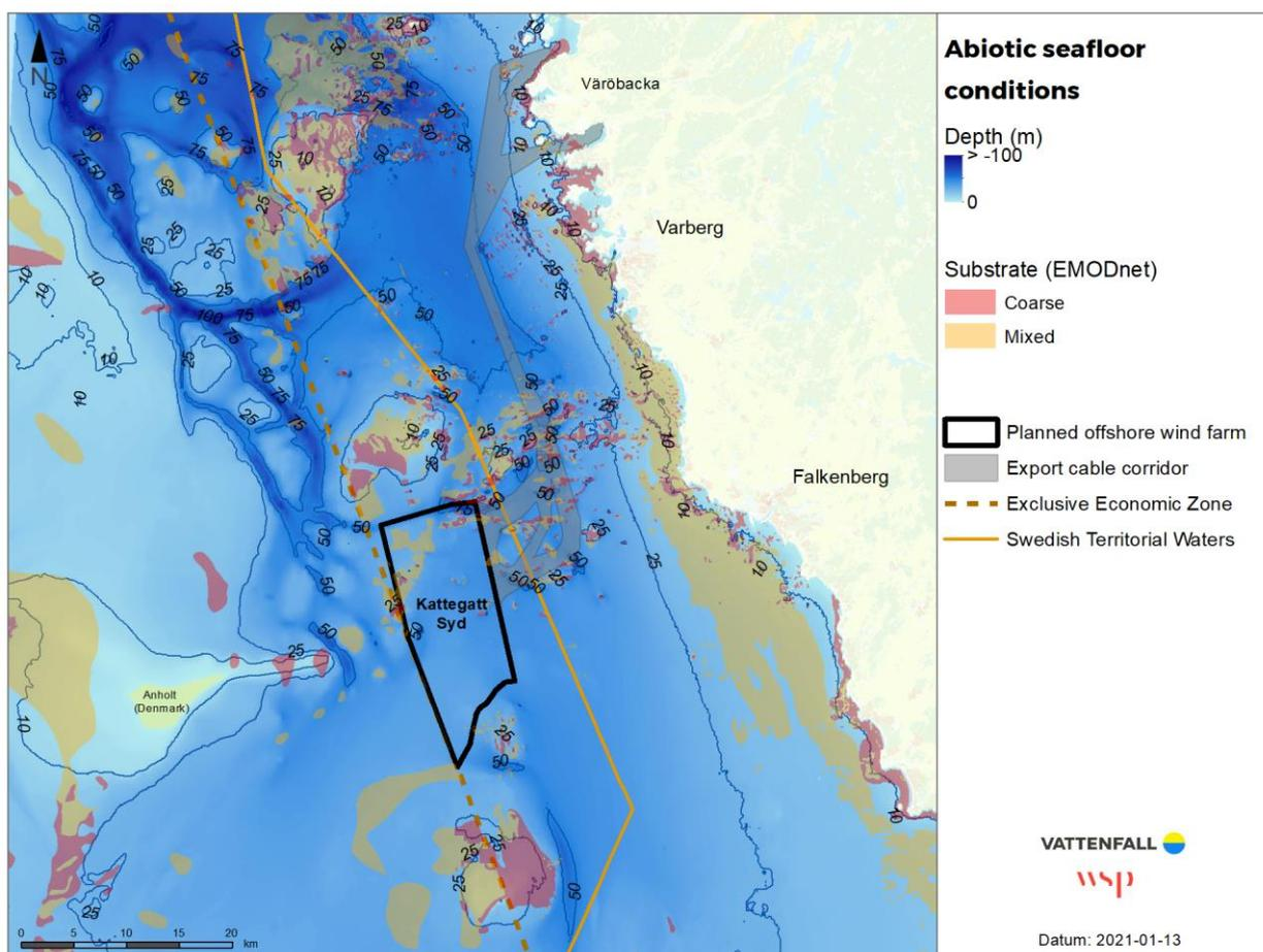
Figure 10. Depth and substrate conditions in the Kattegatt Syd area (data source: EMODnet).
