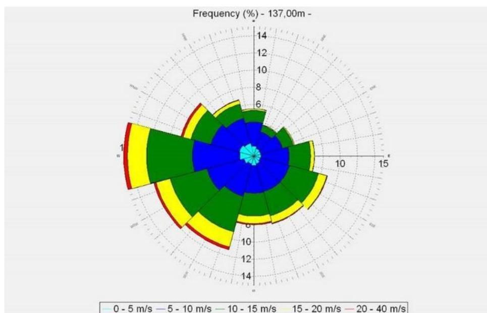
Figure 9. Wind rose for Kattégatt Syd, modelled for 137 m above the mean sea level.
