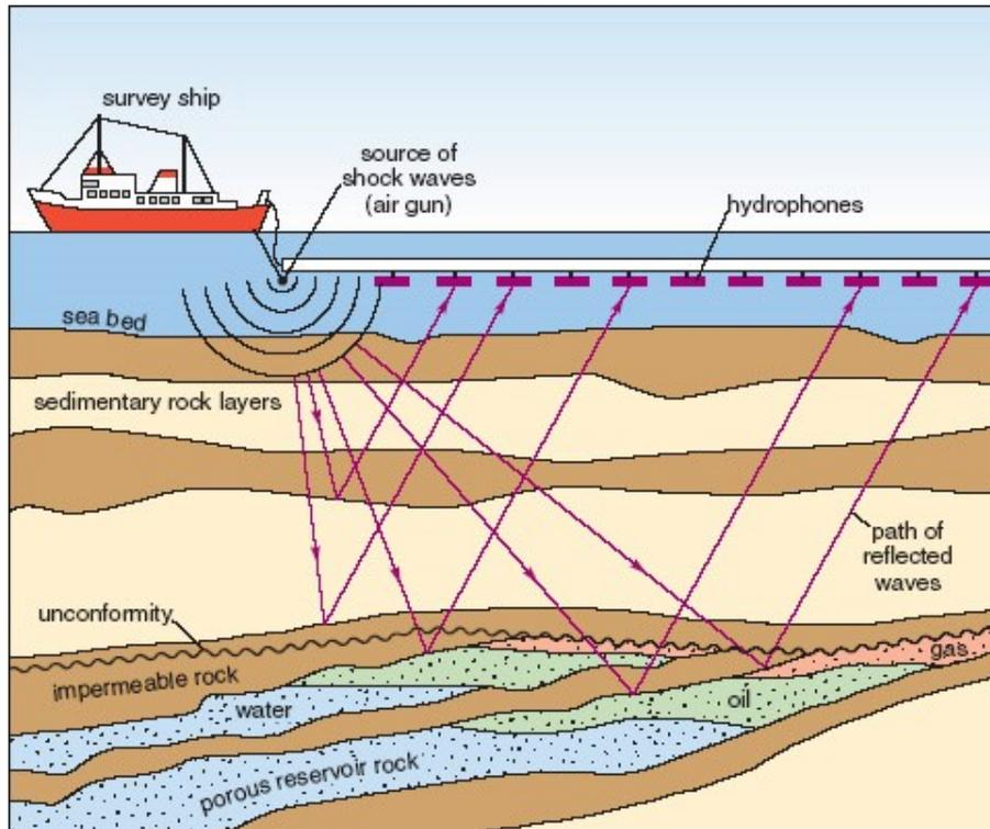
Figure 5 Illustration of a seismic survey. (Image source: <http://openlearn.open.ac.uk/mod/resource/view.php?id=172129>)
