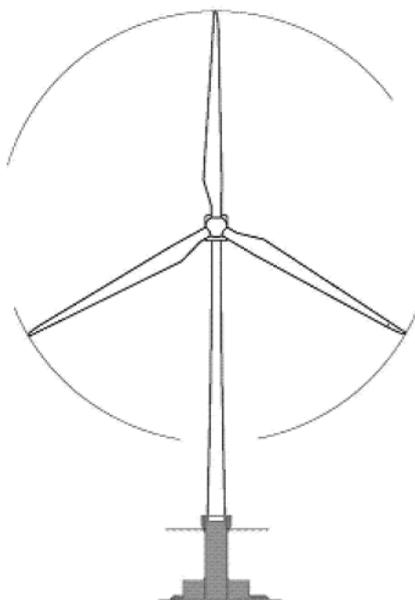
*Figure 11 Wind turbine, basic diagram. The wind turbine is made up of a foundation, a tower with turbine housing and a rotor.*
