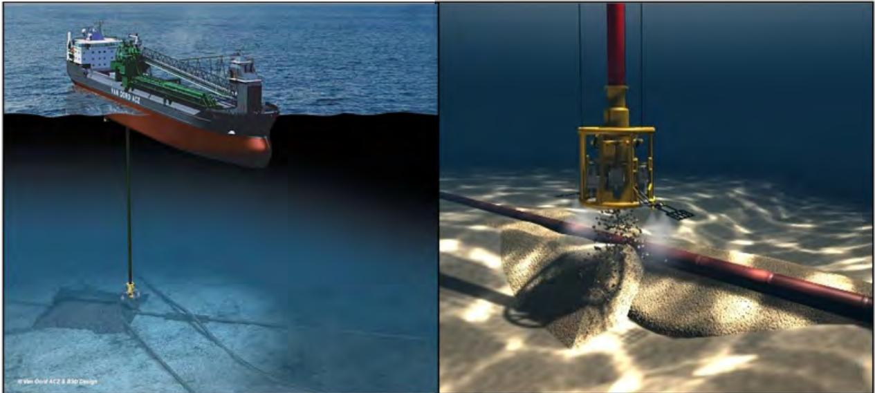
Figure 11: Gravel placement on the seabed through a fall-pipe
