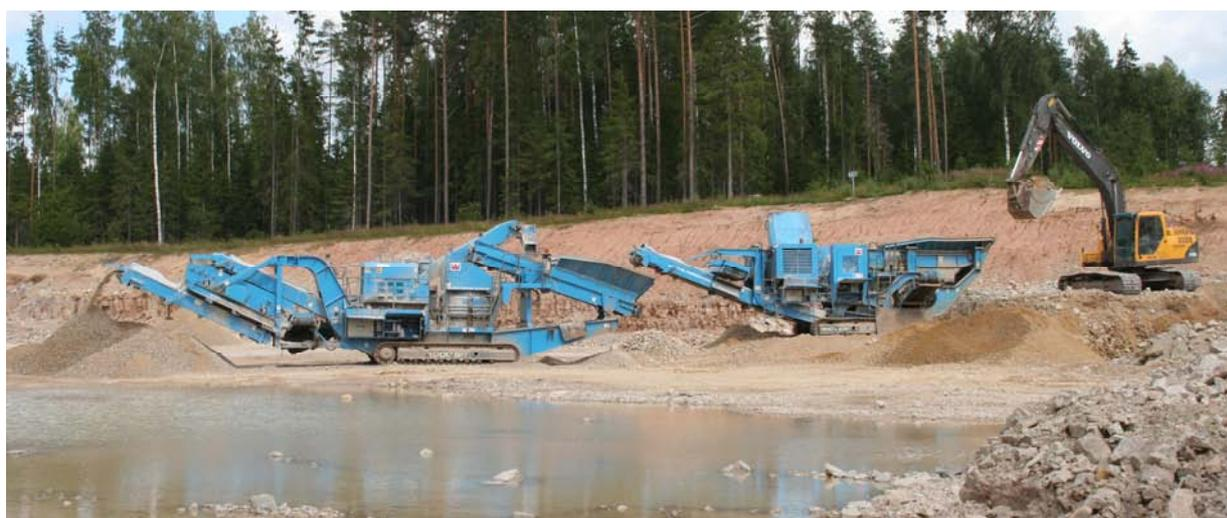
Figure 2. Crushing and screening dolostone at Marinova dolostone quarry in Võru County.
