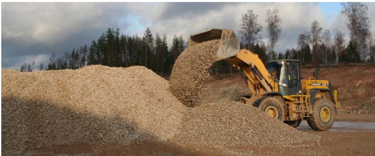
Figure 3. Transport of the aggregate to the piles by a wheeled loader at Marinoa dolostone quarry in Võru County.
