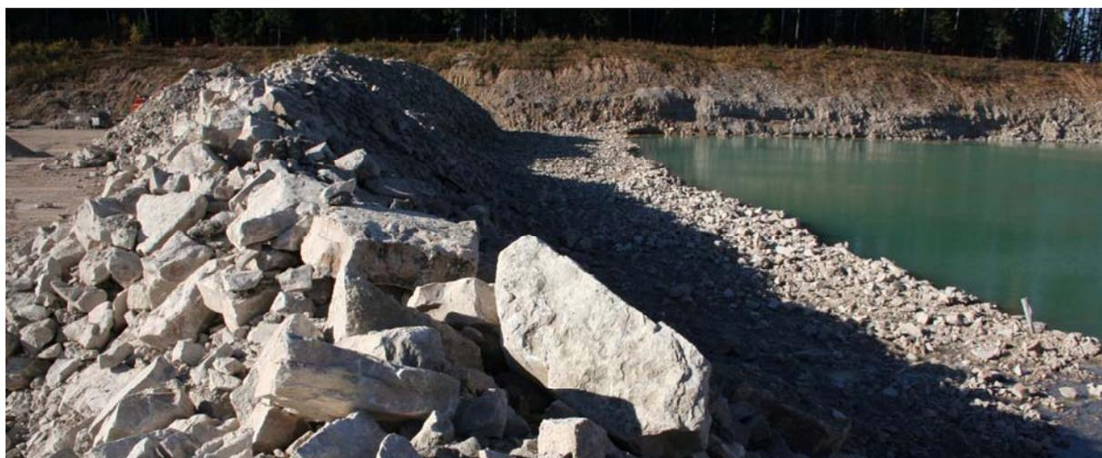
Figure 9. The underwater dolostone in Marinova quarry in Võru County is blasted to a depth of 6 m. On the left, we see the fragmented dolostone lifted from under the water and on the right is the body of water in the quarry.
