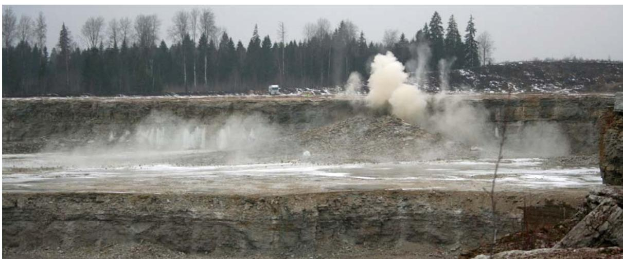
Figure 5. Using blasting to fragment limestone in limestone quarry no. II at Otisaare in Jõgeva County. Photograph taken from 300 m away in the fifth second of the blasting. After the dolostone is fragmented, the dust disperses quickly.
