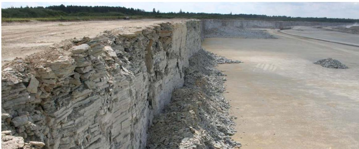
Figure 10. At Aru-Lõuna quarry in Lääne-Viru County, the limestone is blasted “dry,” as the water level has been lowered to the level of the bottom of the quarry. The height of the quarry wall is approximately 15 metres. In the background under the wall, we see how far the pieces of rock are strewn during blasting – up to 50 metres.
