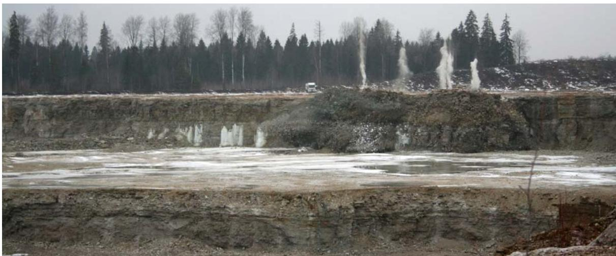
Figure 4. Using blasting to fragment limestone in limestone quarry no. II in Otisaare in Jõgeva County. Photograph taken from 300 m away one second after blasting. The fragmented dolostone flies a few dozen meters in the direction of the quarried area.
