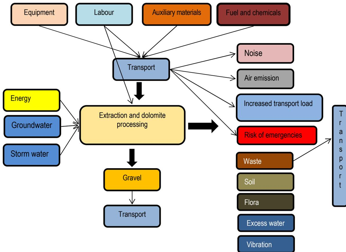
Figure 2. The main inputs and outputs of the quarry operations
