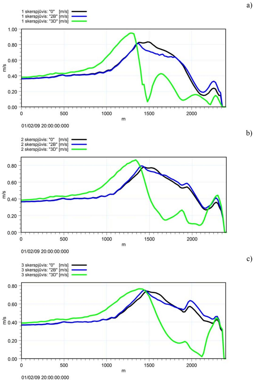
**Fig. 18.** The flow speeds for zero alternative, “2B” and “3D” options in 3 cross-sections (Fig. 12), when SW wind is blowing: 1 (a), 2 (b) and 3 (c) cross-section
