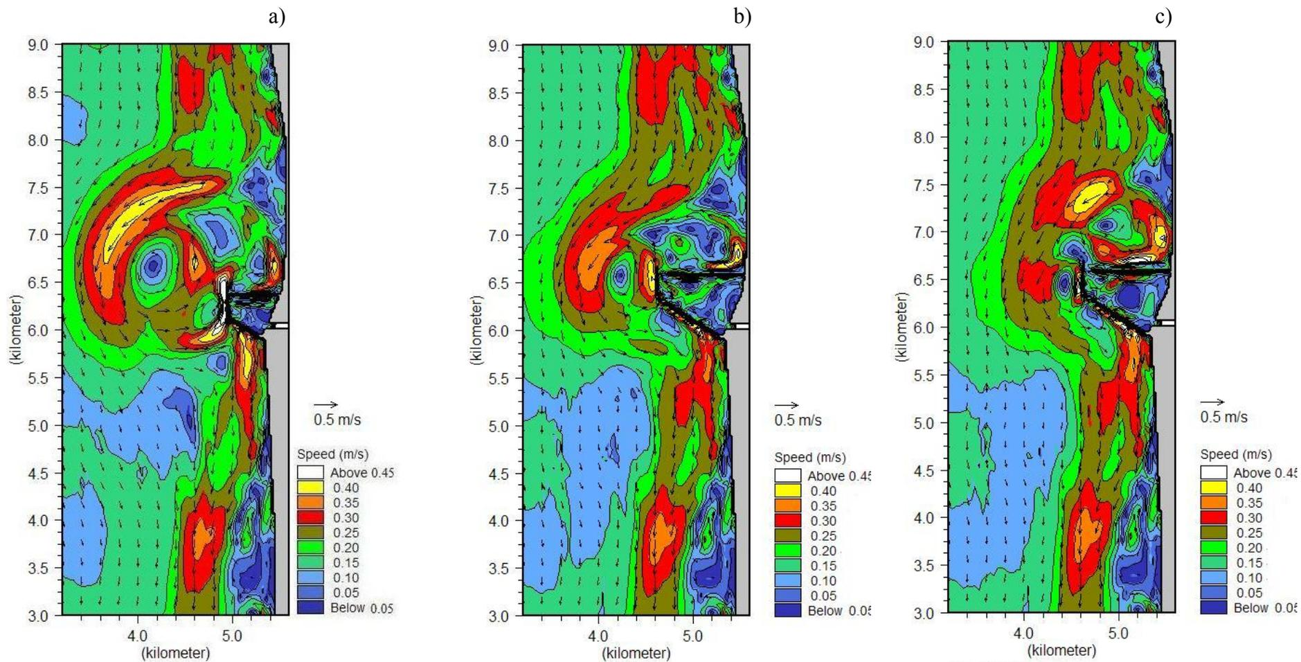
**Fig. 11.** The flow structure, when W wind of 20 m/s speed is blowing: “2C“ (a), “3D“ (b) and “3E“ (c) options
