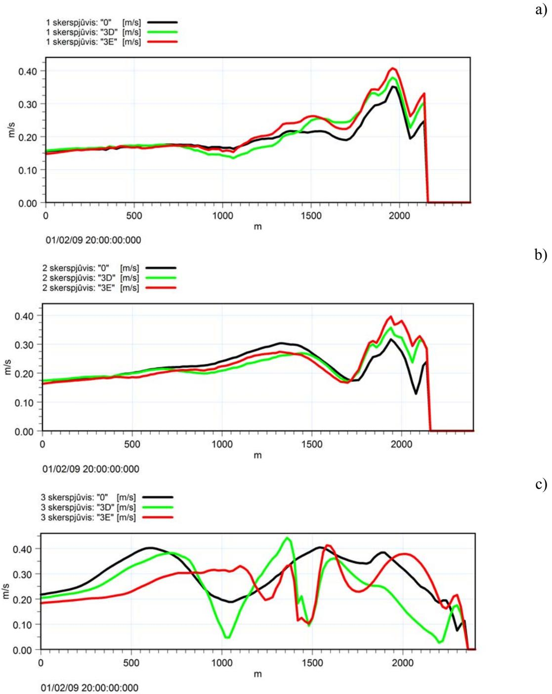
**Fig. 20.** Flow speeds for zero alternative, “3D” and “3E” options (Fig. 10). The blowing wind direction W: 1 (a), 2 (b) and 3 (c) cross-section
