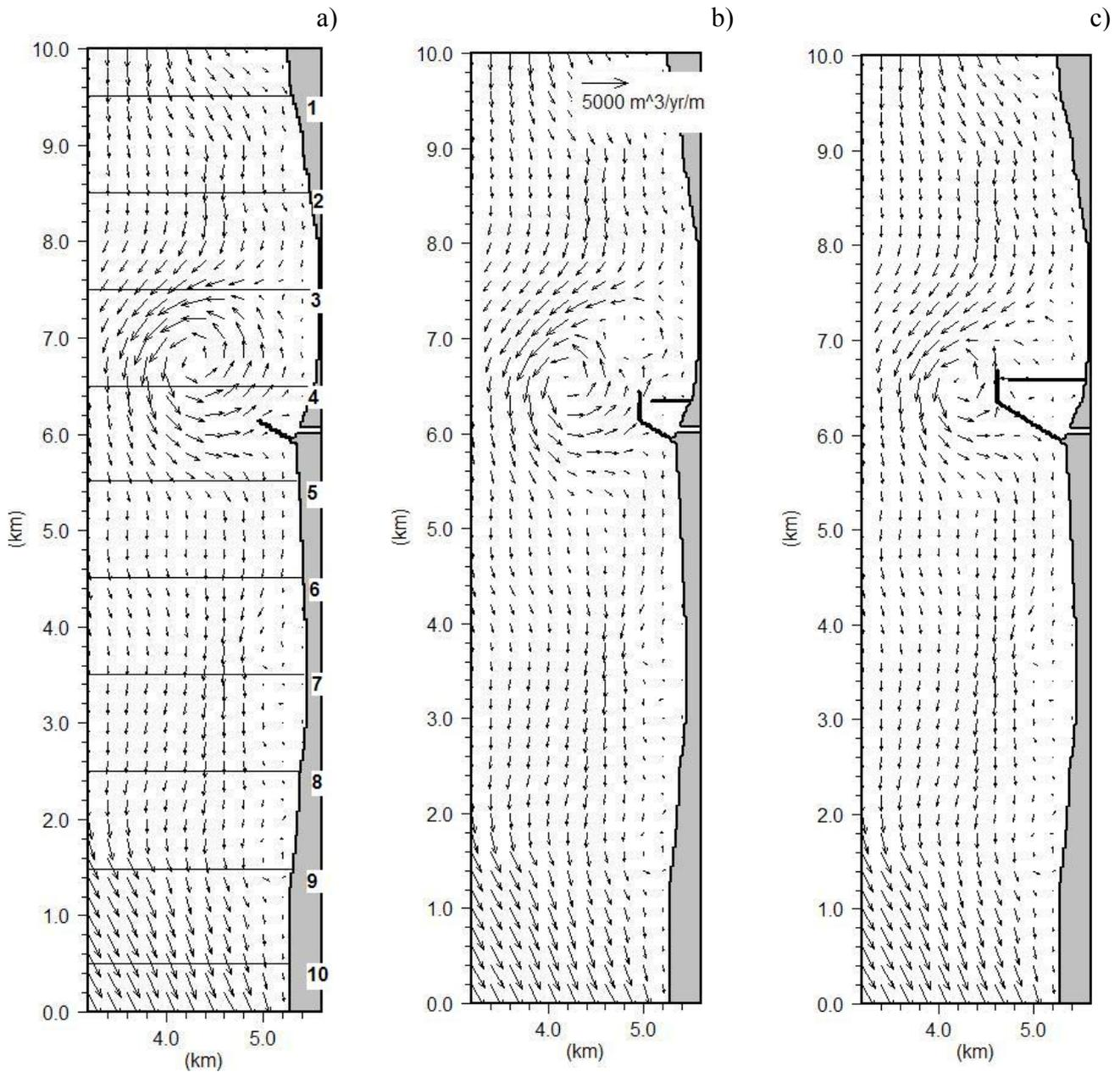
**Fig. 29.** Distribution of the sediment unitary discharge (m<sup>3</sup>/year/m) for W wind with speed 20 m/s for zero alternative, “2B” and “3D” options (calculations of the sediment discharge is done from 10 till 1 cross-section)
