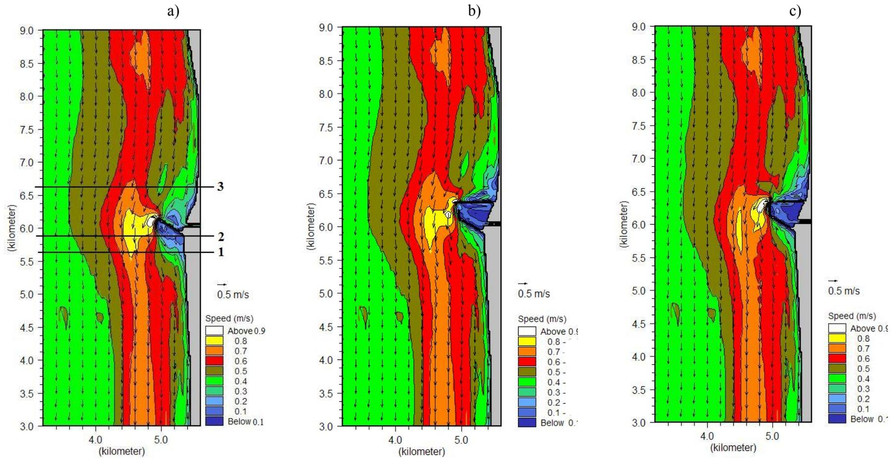
**Fig. 14.** The flow structure, when NW wind of 20 m/s speed is blowing: zero alternative (a), “2A“ (b) and “2B“ (c) options
