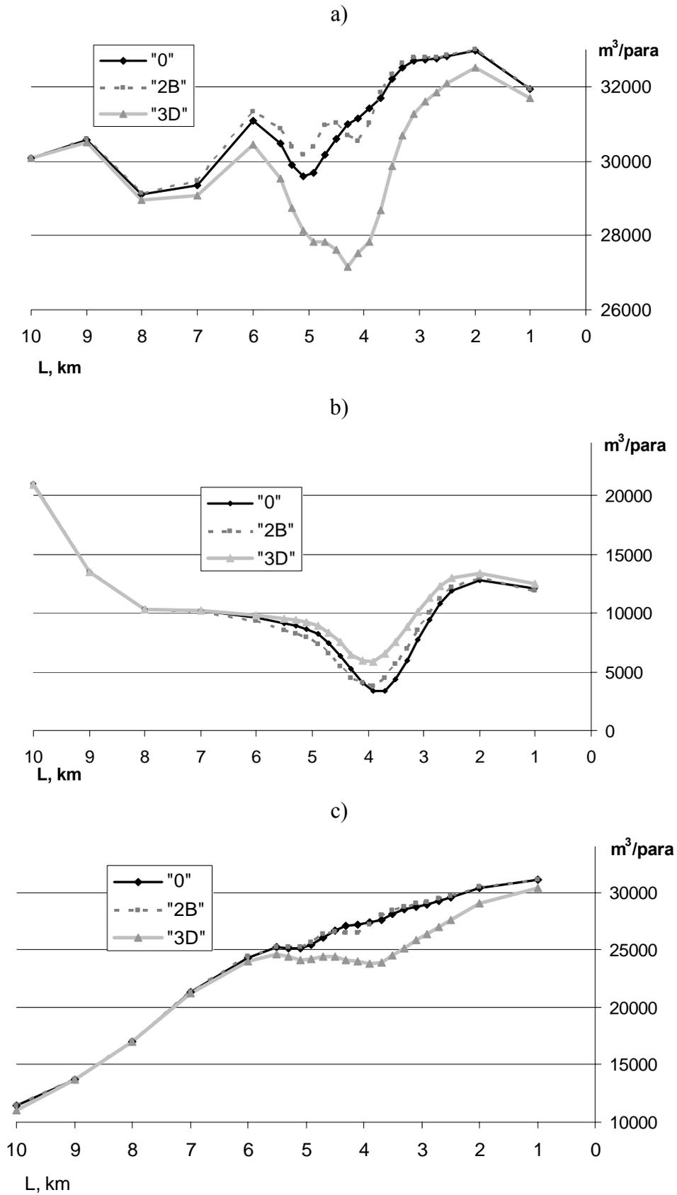
**Fig. 30.** Distribution of the sediment discharge ( $m^3/day$ ) from cross-section 10 (the Ošupis stream) to 1 (1 km to the LT-LV border) for zero alternative, "2B" and "3D" options, for the wind speed 20 m/s and directions NW (a), W (b) and SW (c). Ports breakwaters are between 4 and 5 cross-section
