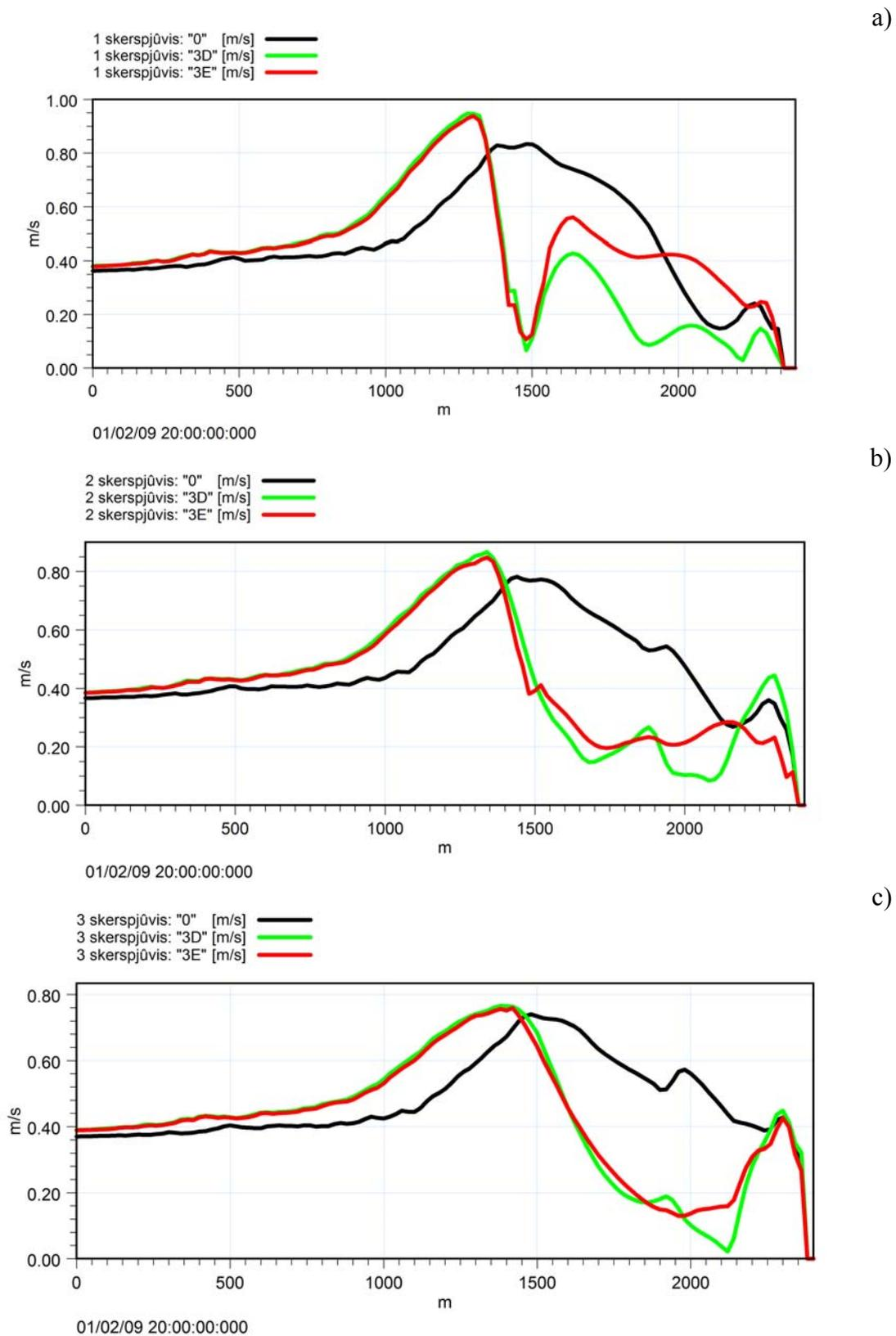
**Fig. 22.** Flow speeds for zero alternative, “3D” and “3E” options for the three cross-sections (Fig. 12). The blowing wind direction SW: 1 (a), 2 (b) and 3 (c) cross-section
