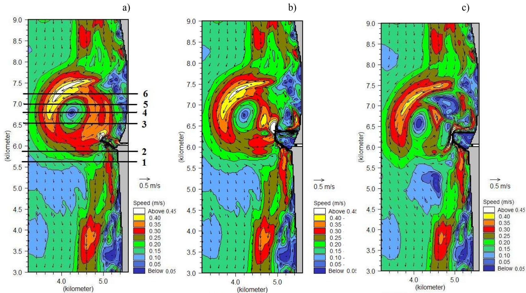
**Fig. 10.** The flow structure, when W wind of 20 m/s speed is blowing: zero alternative (a), “2A“ (b) and “2B“ (c) options
