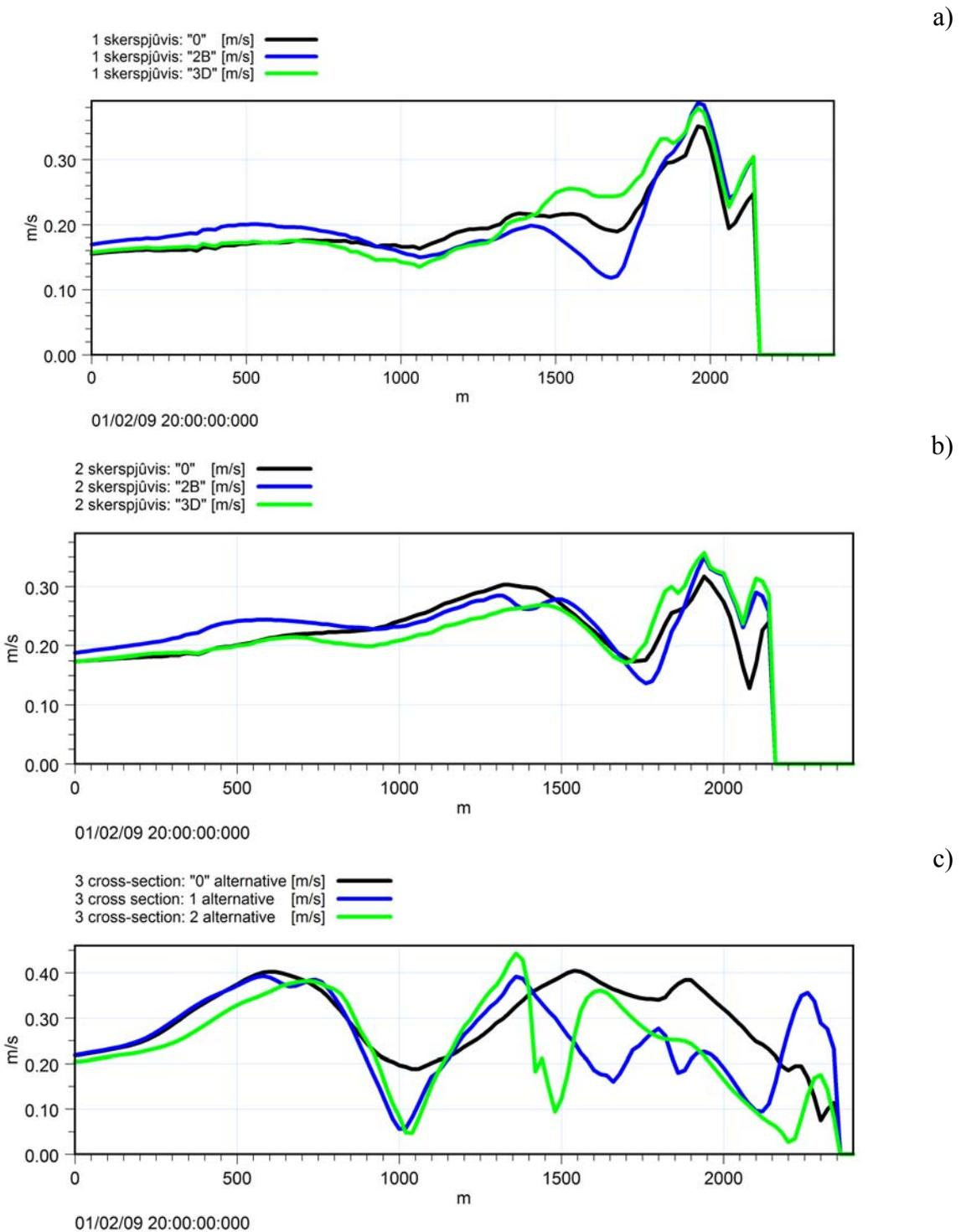
**Fig. 16.** The flow speeds for zero alternative, “2B” and “3D” options in 3 cross-sections (Fig.10), when W wind is blowing: 1 (a), 2 (b) and 3 (c) cross-section
