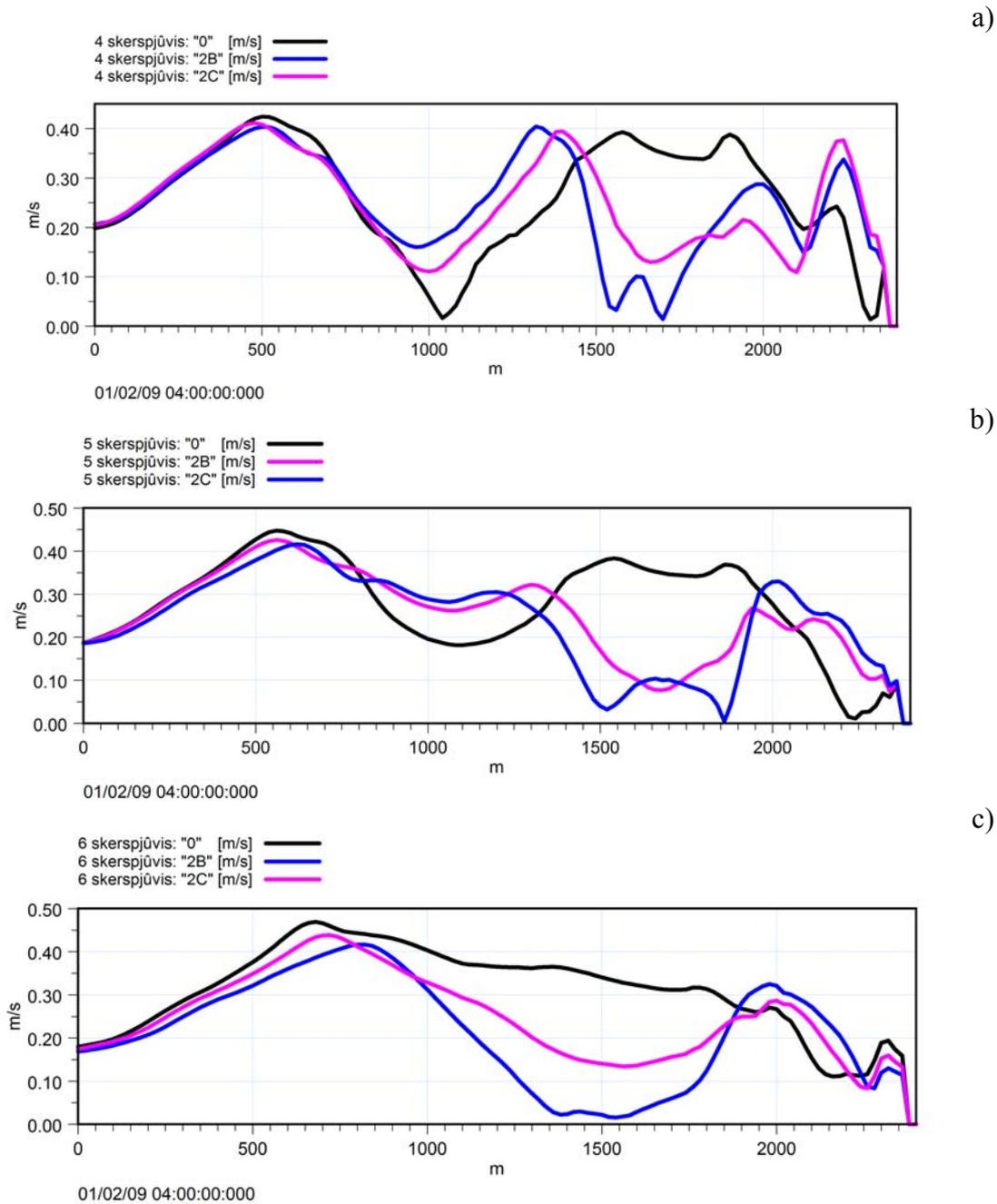
**Fig. 25.** Flow speeds for zero alternative, “2B” and “2C” options in the three cross-sections (Fig. 10). The blowing wind direction W: 4 (a), 5 (b) and 6 (c) cross-sections
