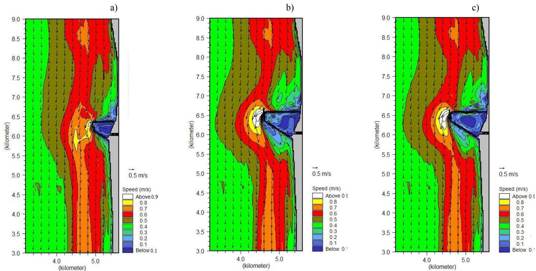
**Fig. 15.** The flow structure, when NW wind of 20 m/s speed is blowing: “2C” (a), “3D” (b) and “3E” (c) options
