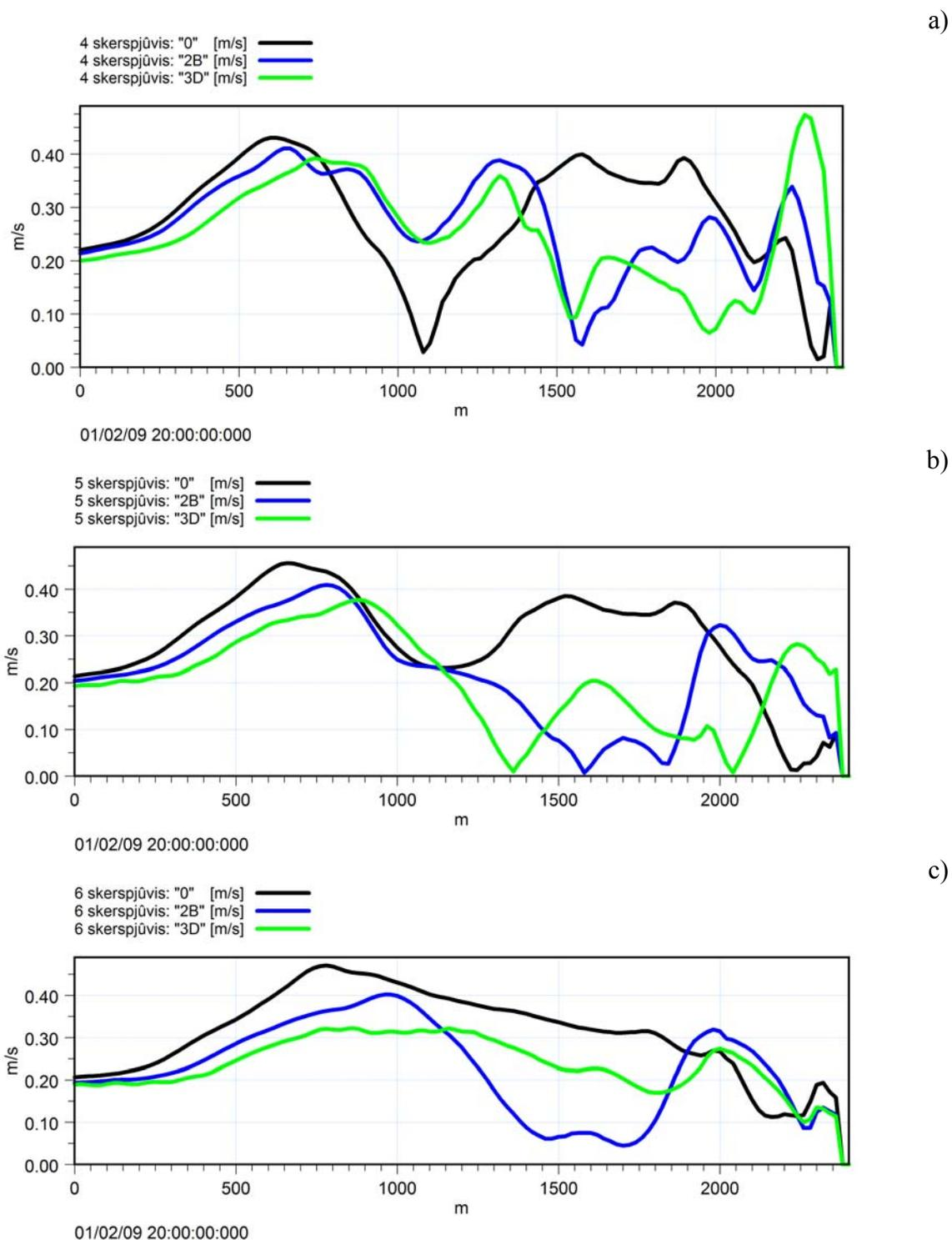
**Fig. 17.** The flow speeds for zero alternative, “2B” and “3D” options in 3 cross-sections (Fig. 10), when W wind is blowing: 4 (a), 5 (b) and 6 (c) cross-section
