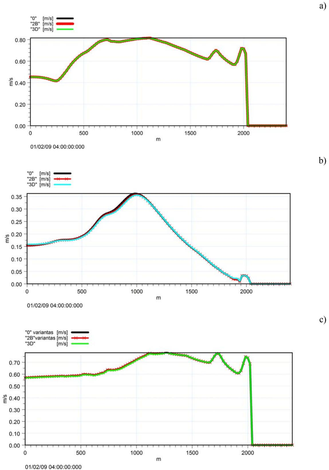
**Fig. 28.** Flow speeds for zero alternative, "2B" and "3D" options in the cross-section, which is situated 5 km from the Šventoji breakwater to the north (Latvian territory), for the wind directions NW (a), W (b) and SW (c). Cross-section starts (0) at the sea and ends at the mark 2050 m
