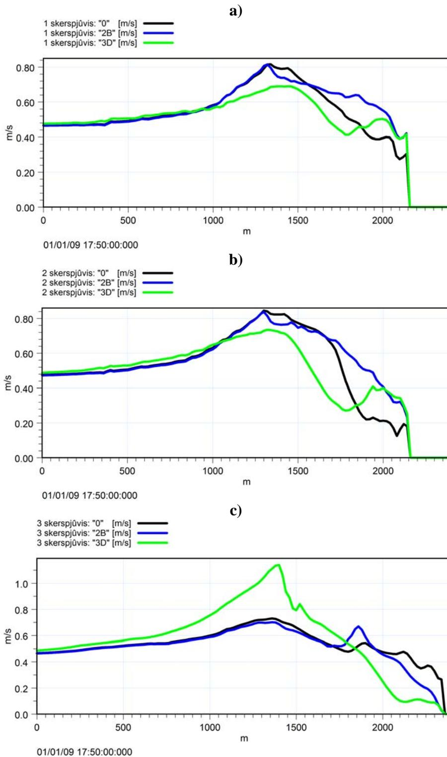
**Fig. 19.** The flow speeds for zero alternative, “2B” and “3D” options in 3 cross-sections (Fig. 14), when NW wind is blowing: 1 (a), 2 (b) and 3 (c) cross-section
