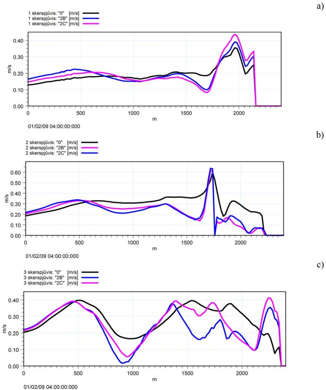
**Fig. 24.** Flow speeds for zero alternative, "2B" and "2C" options in the three cross-sections (Fig. 10). The blowing wind direction W: 1 (a), 2 (b) and 3 (c) cross-section
