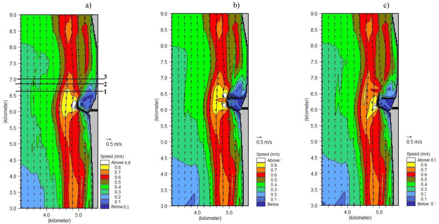
**Fig. 12.** The flow structure, when SW wind of 20 m/s speed is blowing: zero alternative (a), “2A” (b) and “2B” (c) options
