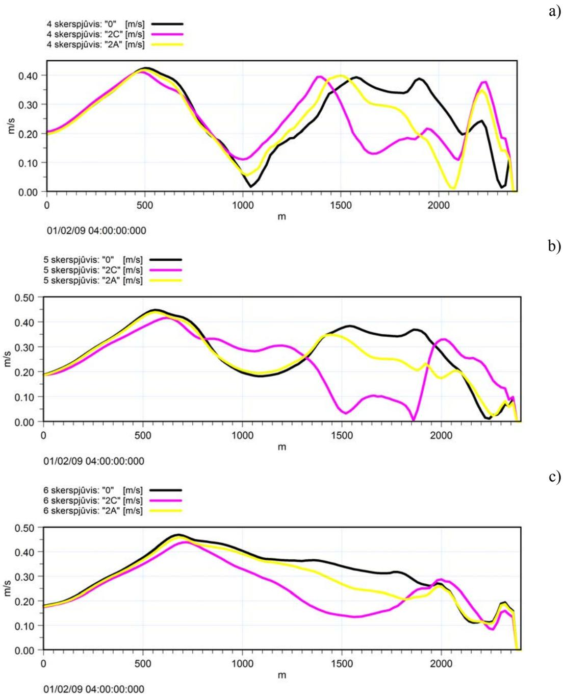
**Fig. 27.** Flow speeds for zero alternative, “2C” and “2A” options in the three cross-sections (Fig. 10). The blowing wind direction W: 4 (a), 5 (b) and 6 (c) cross-sections
