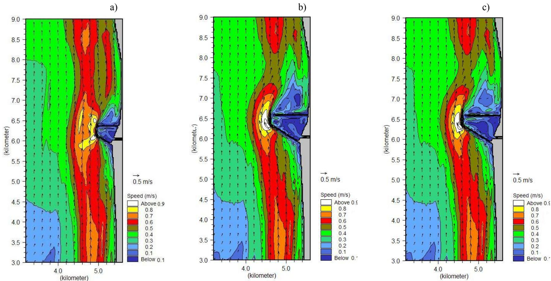
**Fig. 13.** The flow structure, when SW wind of 20 m/s speed is blowing: “2C“ (a), “3D“ (b) and “3E“ (c) options
