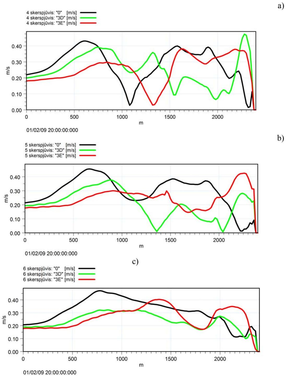
**Fig. 21.** Flow speeds for zero alternative, "3D" and "3E" options for the three cross-sections (Fig. 10). The blowing wind direction W: 4 (a), 5 (b) and 6 (c) cross-section
