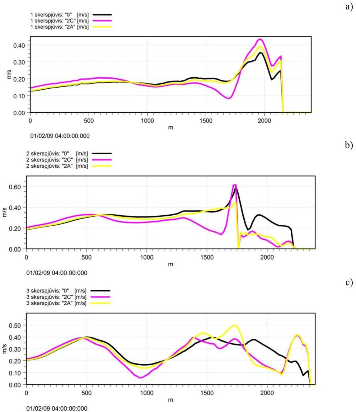
**Fig. 26.** Flow speeds for zero alternative, “2C” and “2A” options in the three cross-sections (Fig. 10). The blowing wind direction W: 1 (a), 2 (b) and 3 (c) cross-sections
