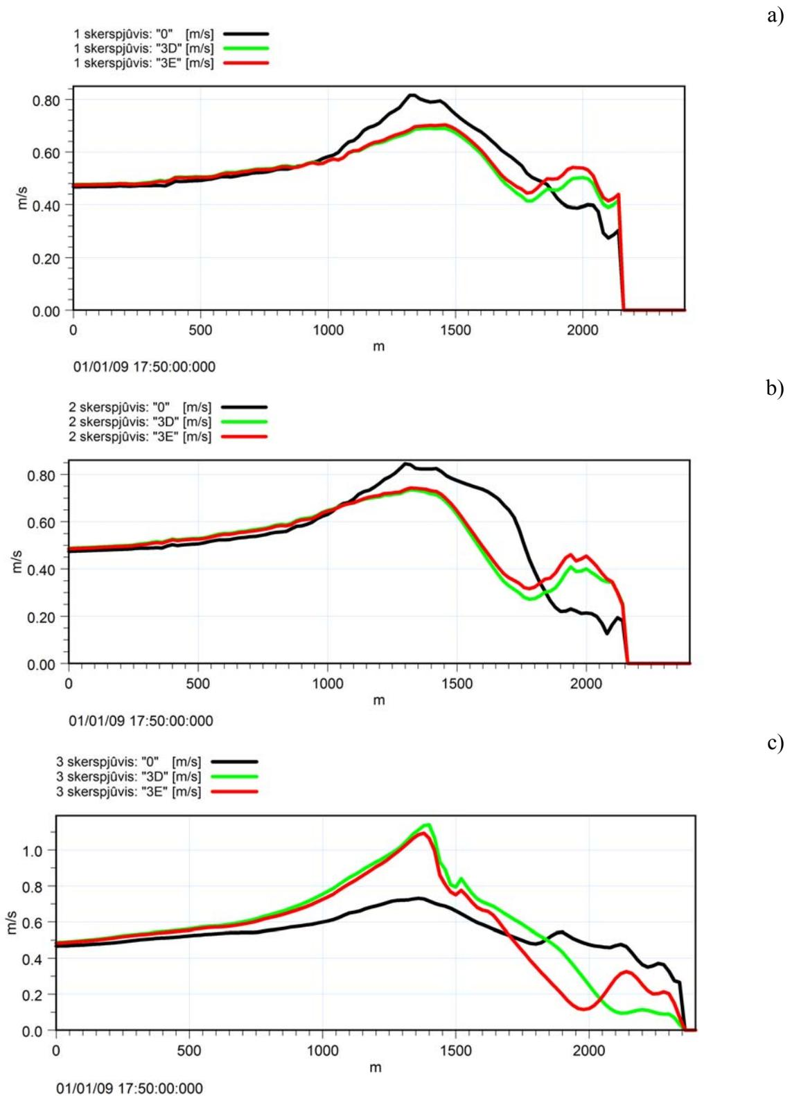
**Fig. 23.** Flow speeds for zero alternative, “3D” and “3E” options for the three cross-sections (Fig. 14). The blowing wind direction NW: 1 (a), 2 (b) and 3 (c) cross-section
