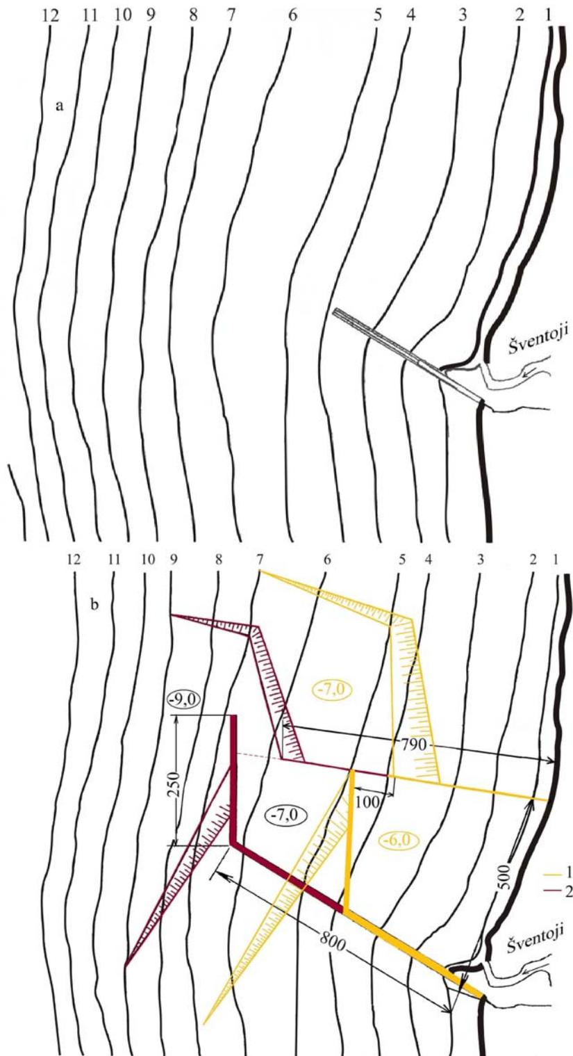
**Fig. 2.** Zero alternative of the Šventoji State Sea Port reconstruction (a) and option “2B” (b) with opportunity to extend breakwaters and to deepen the entrance channel according to option “3E”. 1 – option “2B”, 2 – option “3E”
