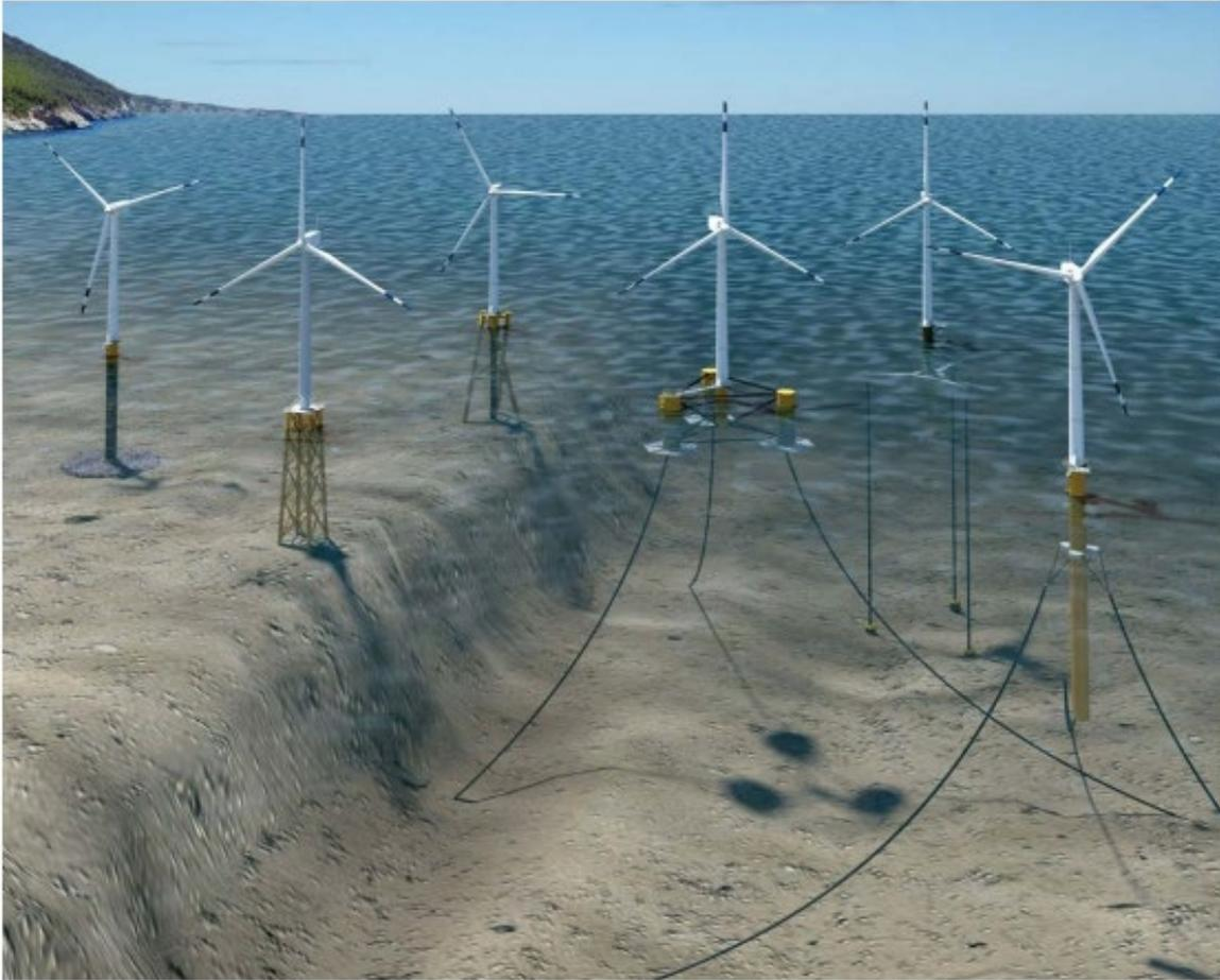
Figure 7. Different types of foundations: from the left: monopile, jack, IBGS, semi-submersible, TLP and SPAR buoy, (NREL 2014-2015 Offshore Wind Technologies Market Report).
