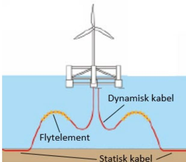
Figure 12. Principle sketch internal cable mesh for floating foundations.
