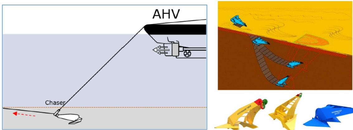
Figure 10. Installation of drag embedded anchors (Mooring System Engineering).
