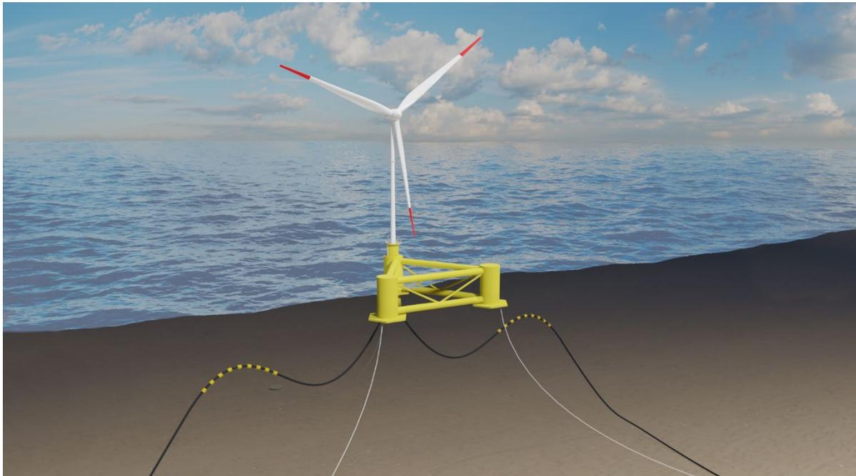
*Figure 8. Generic semi-submersible platform, with wind turbine, anchorage and internal electrical cables (Deep Wind Offshore/Norconsult, 2021).*
