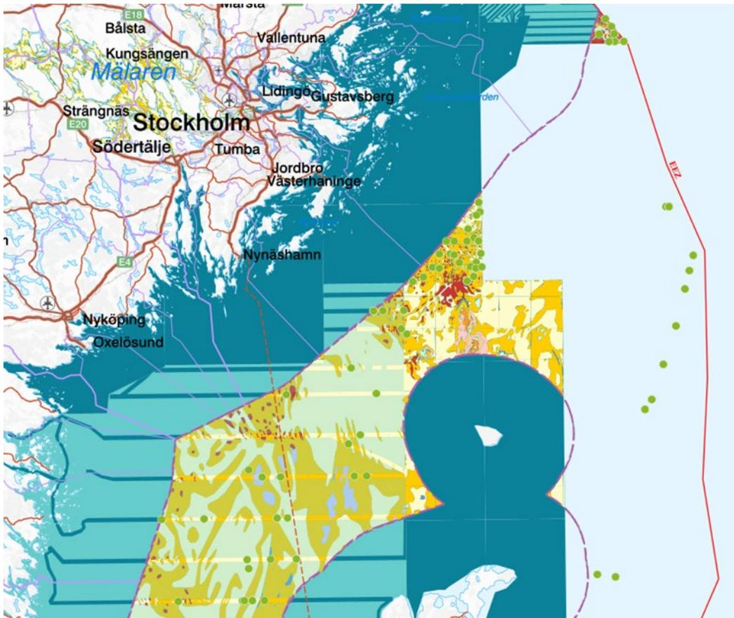
Figure 15. Seabed conditions within the area in question - orange/yellow parts represent different types of clay sediments in the bottom layer (Geological Survey of Sweden, 2022).
