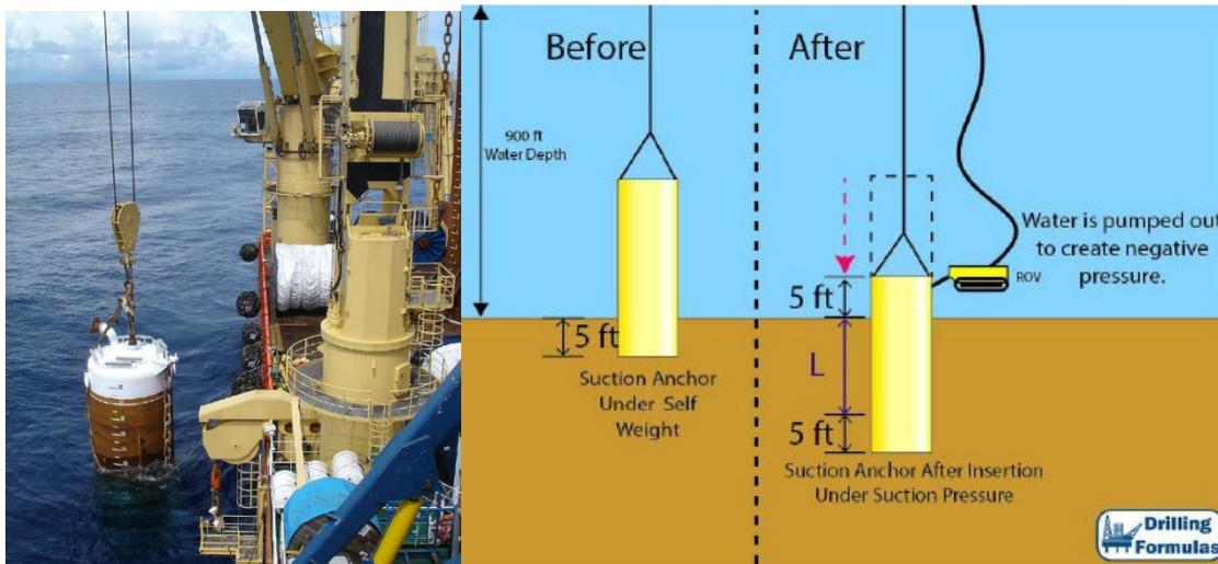
Figure 9. Installation of suction anchors (Drilling Formulas).
