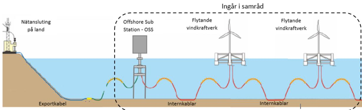
Figure 5. Outline of principles for different parts of an offshore wind farm and which parts are covered by the consultation.
