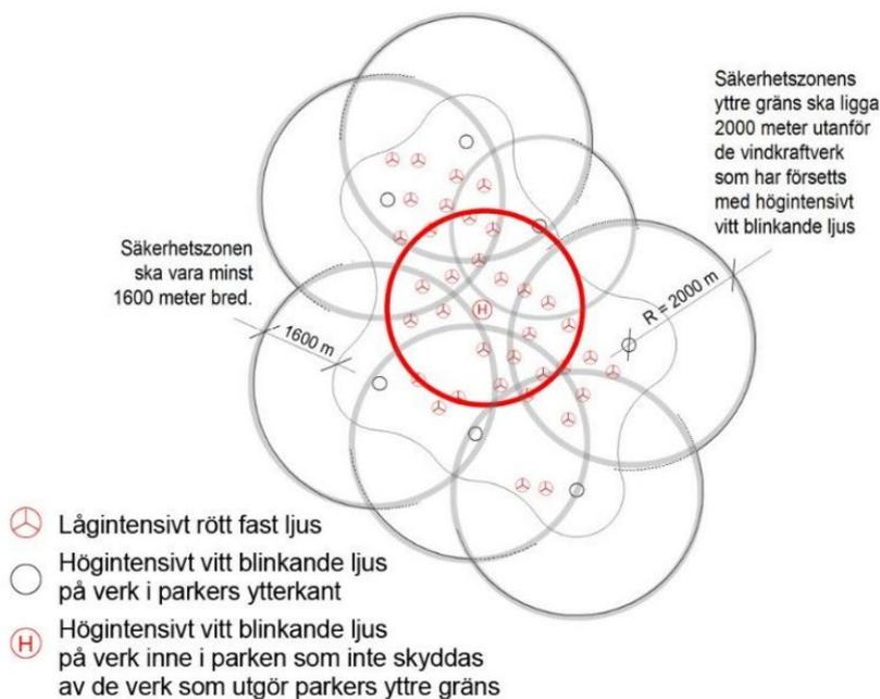
Figure 13. Principle sketch for marking of wind turbines with a total height above 150 metres (TSFS 2020:88).
