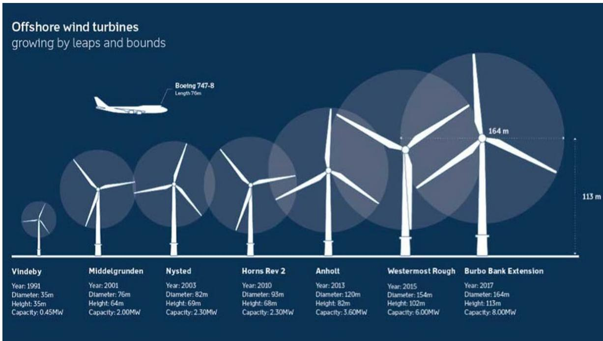
Figure 6. The development of wind turbines in size historically (Open Ocean, 2017).
