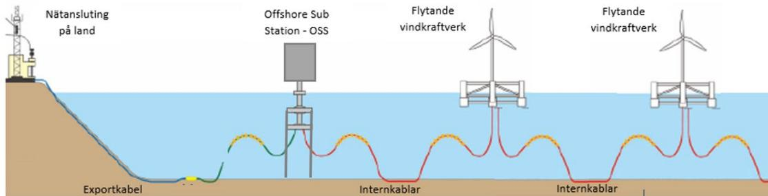
Figure 11. Principle sketch electricity transmission from offshore wind power to onshore. The picture is the same as Figure 5.
