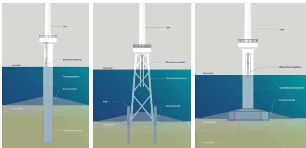
Figure 5. Types of foundations that may be used for the planned wind farm. From left to right; monopile foundations, truss foundations and gravity foundations. (Source: RWE)
