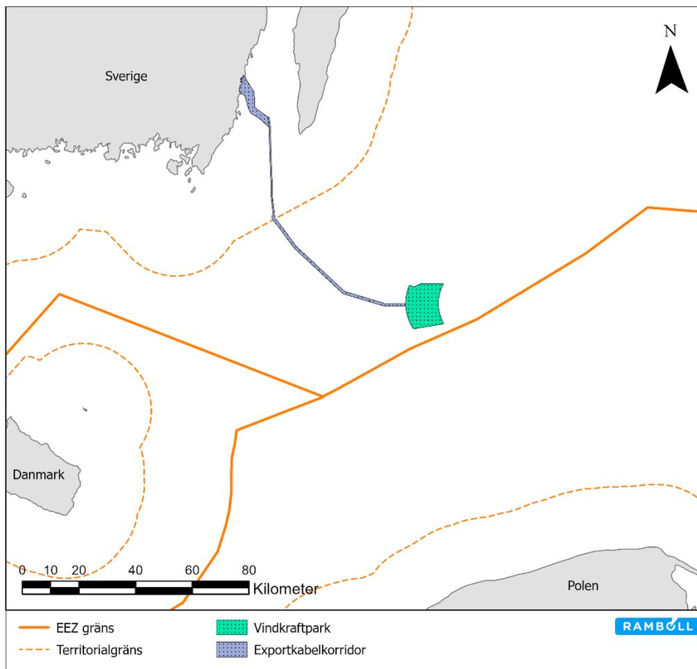
Figure 7. The planned wind farm including the cable corridor for the export cable to land.
