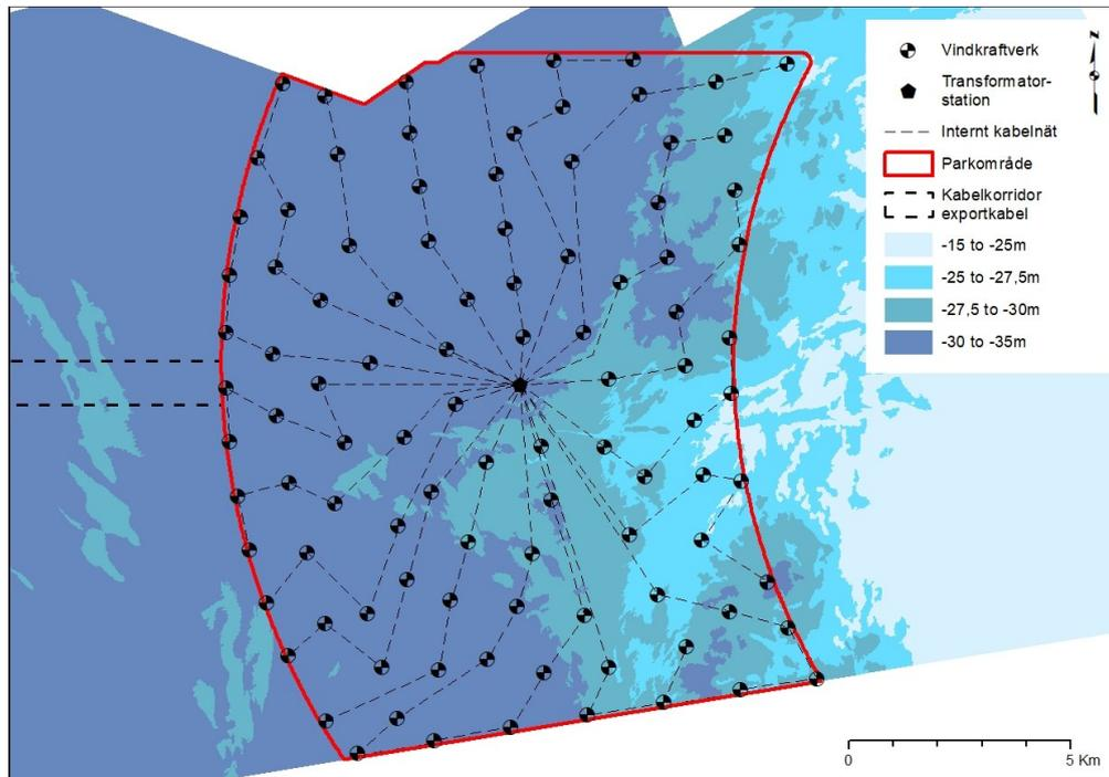
Figure 3. Example layout of the planned wind farm with 100 wind turbines, a centrally located transformer substation and internal cable network.
