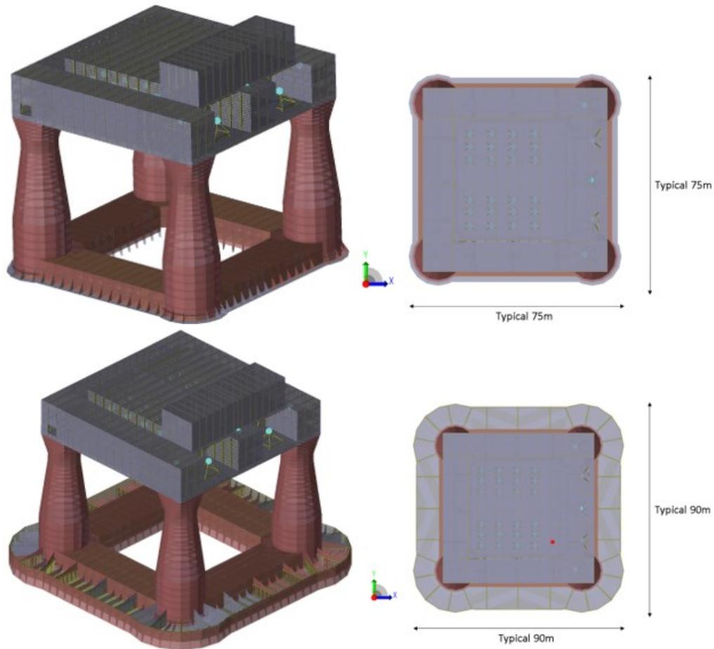
Figure 6. There are two possible concepts for the gravity foundation; supplied complete with ballast placed in the bottom part (top picture) or supplied without ballast in the form of a bottom part with a "balcony" (bottom picture). The foundation is put in place and then the "balcony" is filled with ballast. (Source: RWE)
