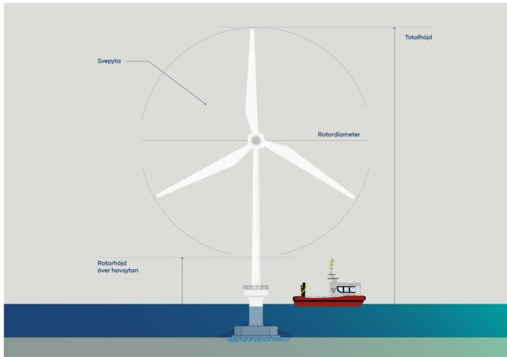
Figure 4. Outline drawing of a wind turbine. (Source: RWE)
