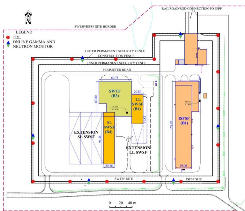
Fig. 4.1-13 Layout of TLD, gamma and neutron dosimeters on the ISFSF/SWTSF sites
