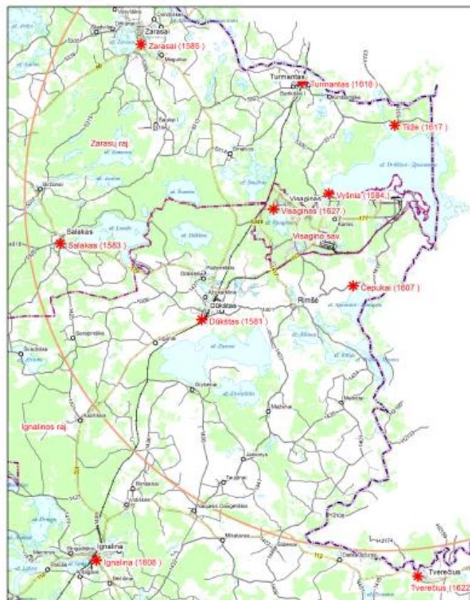
Fig. 4.1-11 Layout of the Skylink system gamma detectors within the INPP 30 km zone
