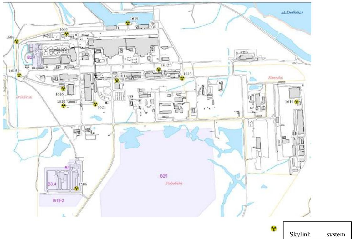
Fig. 4.1-10 Layout of the Skylink system gamma detectors within the INPP 3 km zone
