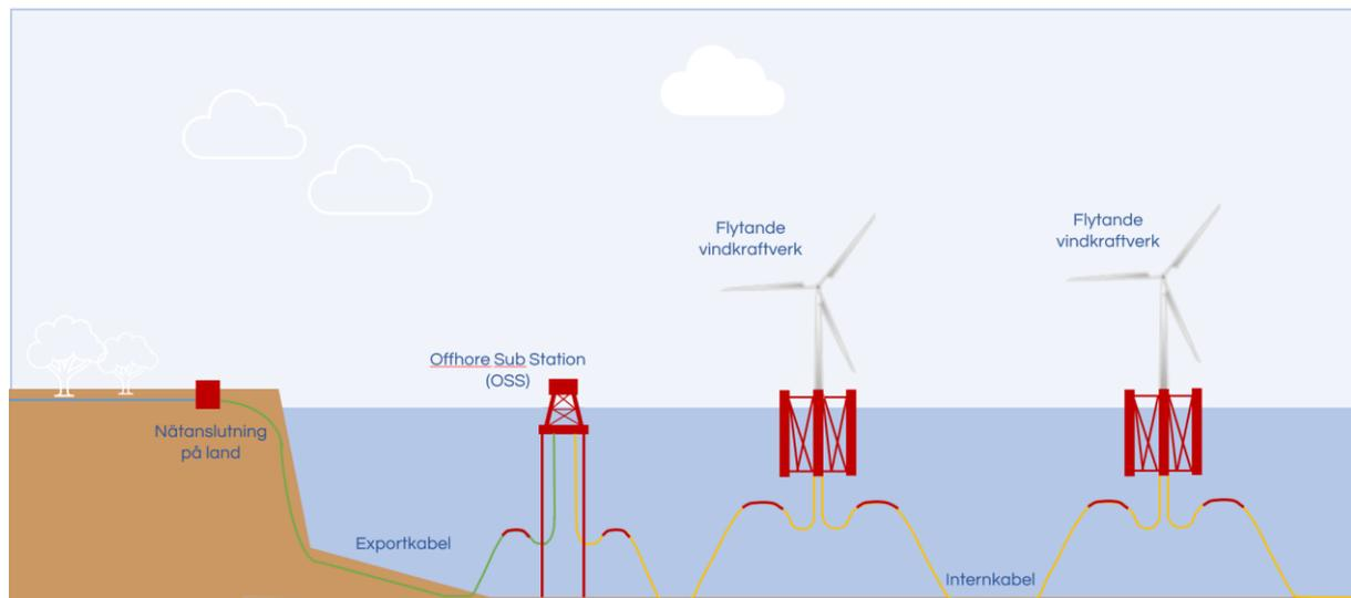
Figure 10. Schematic of the different parts of an offshore wind farm. Nätanslutning på land – Gridconnection on land; Exportkabel - Exportcable; OOS – Offshore Sub Station; Flytande vindkraftverk – Floating wind turbines; Internkabel – Internal cable network.
