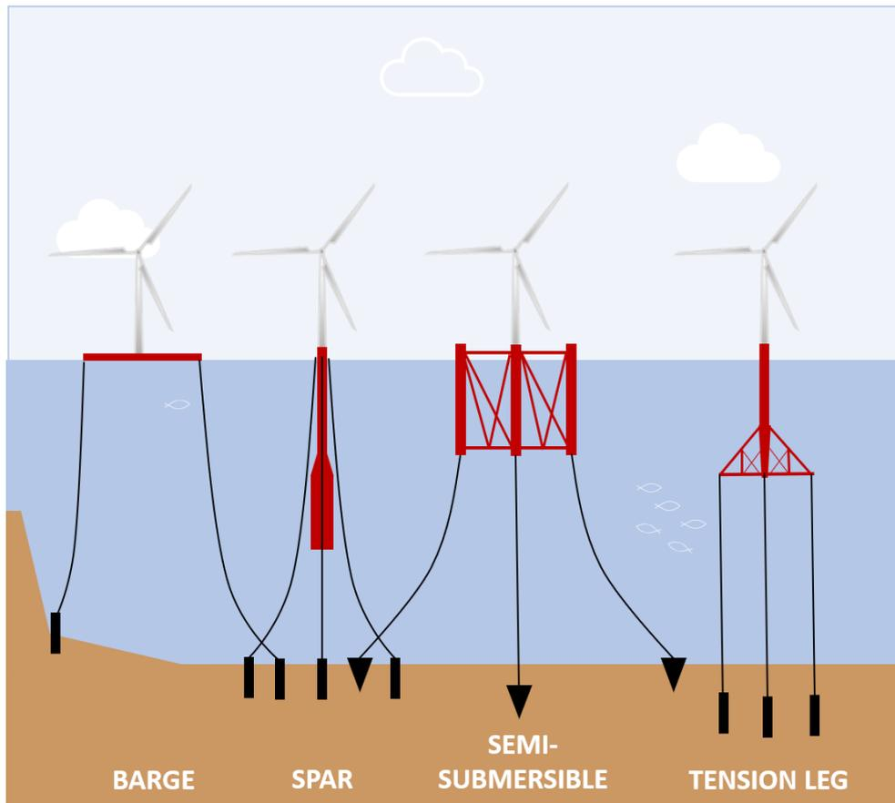
Figure 9. Illustration of the current main models of floating foundations.
