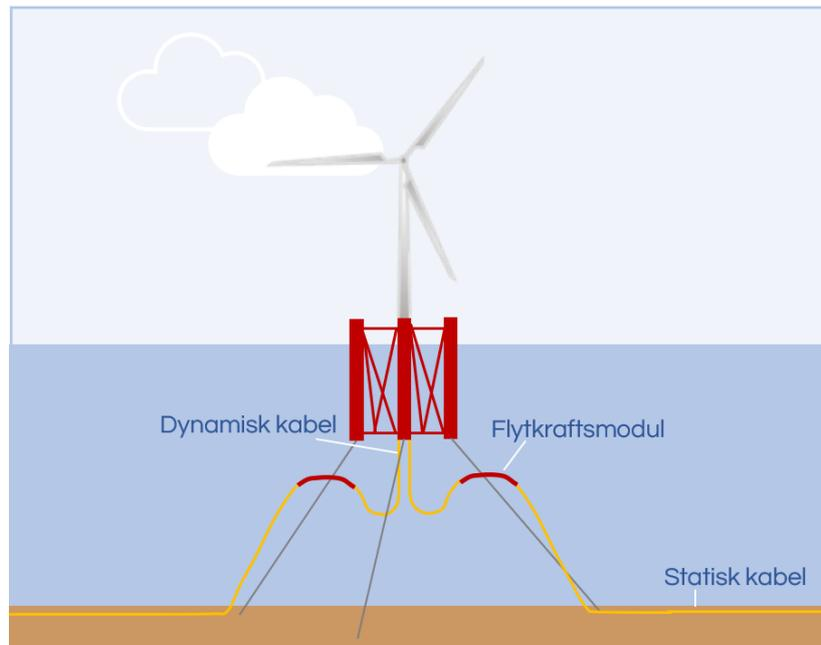
Figure 11. Schematic of the internal cable network. *Dynamisk kabel* – Dynamic cable; *Flytkraftsmodul* - buoyancy module; *Statisk kabel* – Static cable.
