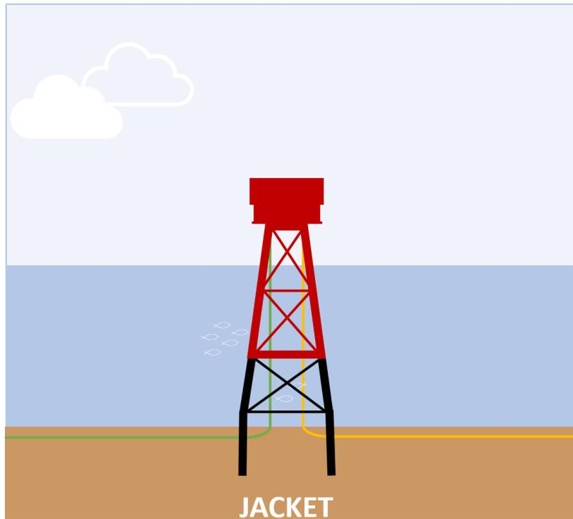
Figure 12. Schematic of a jacket foundation.
