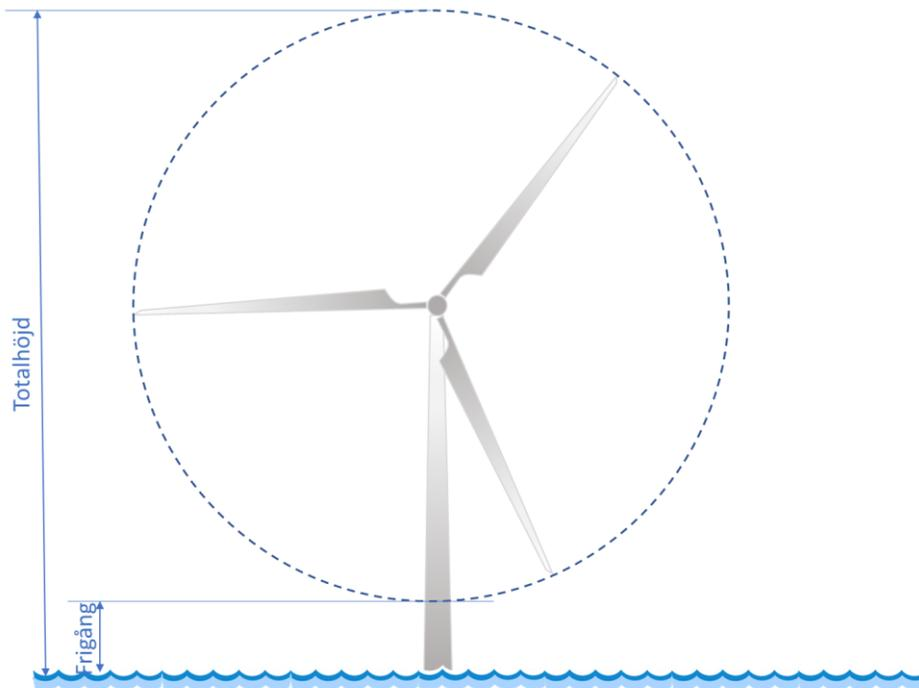
Figure 6. Schematic of example. Frigång – Clearance; Totalhöjd – Total height.
