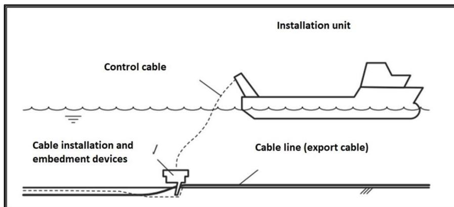
Figure 3.11. Cable line laying technology – burial of a cable previously laid on the seabed (Source: <https://rules.dnv.com>)
