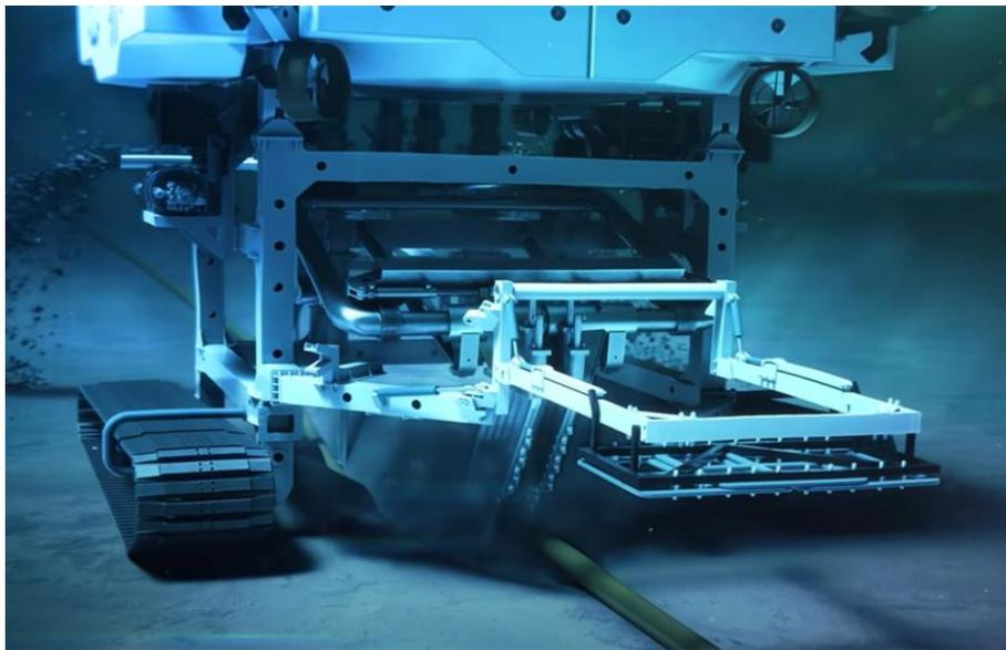
Figure 3.10. Jetting equipment example (Source: <https://www.youtube.com/watch?v=wb1le4zRA2M>)
