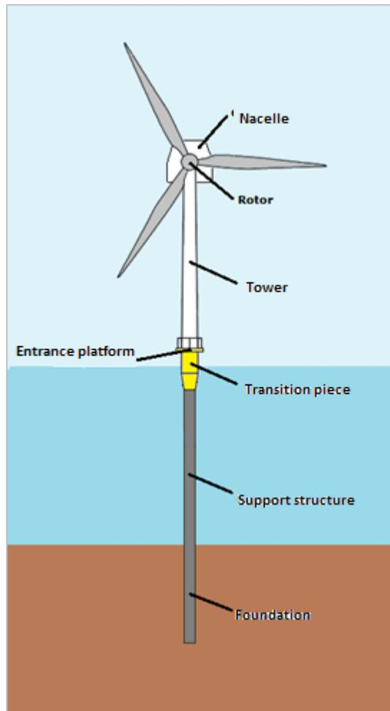
Figure 3.4. Schematic diagram of a single wind turbine with an example of a monopile foundation (source: internal materials)
