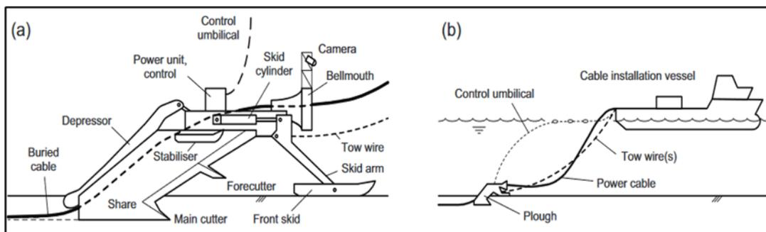
Figure 3.15. Technology of cable line laying using a cable plough (source: <https://rules.dnv.com/>)
