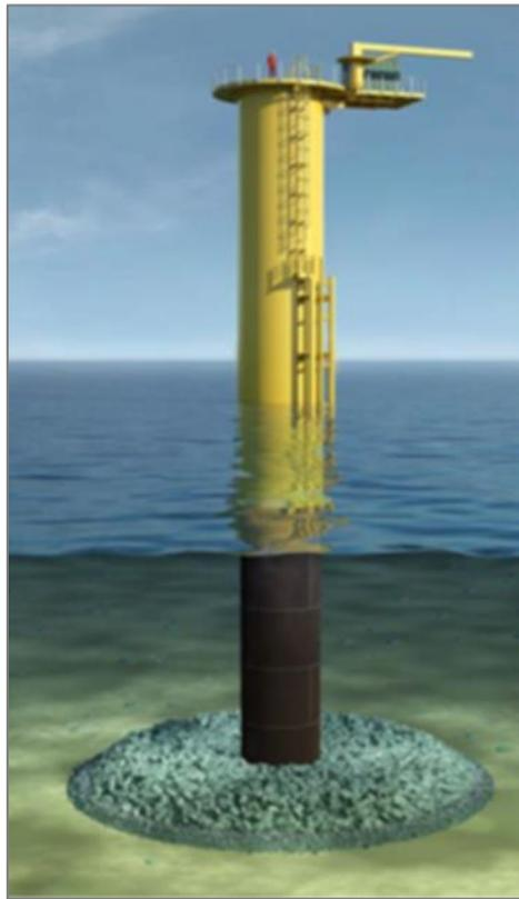
Figure 3.5. Example of a monopile foundation including a scour protection layer (source: Ramboll)
