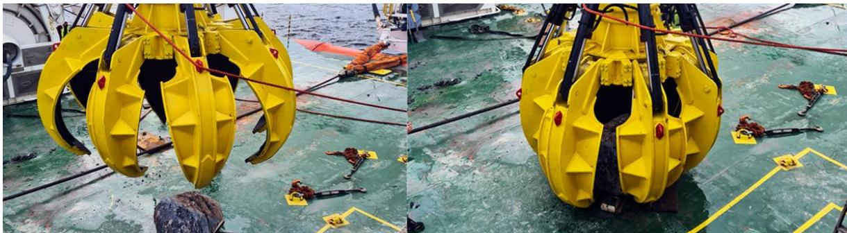
Figure 3.2. Example of a grapple used to remove boulders from the seabed (source: <https://www.assogroup.com/>)
