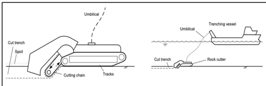
Figure 3.13. Mechanical dredger (source: <https://rules.dnv.com>)
