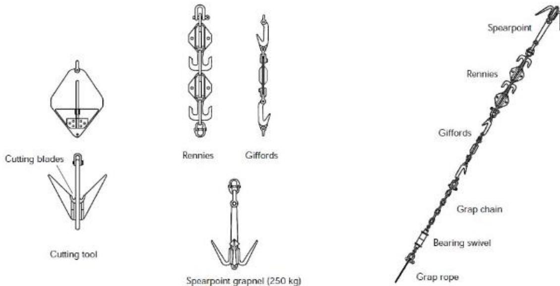
Figure 3.3. Examples of dragged tools for the seabed pre-lay clearance (source: HKA Submarine Cable -Chung Hom Kok, Project Profile)
