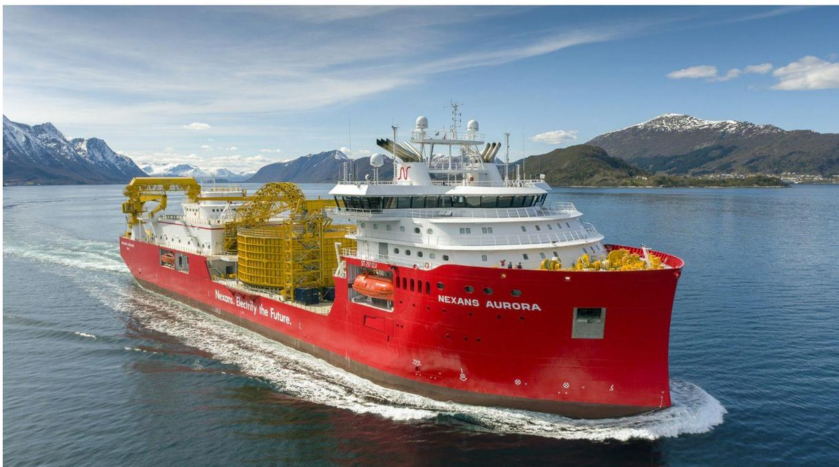
Figure 3.9. Example of a cable layer conducting complex operations related to the laying of subsea cable lines (source: <https://www.nexans.com/>)
