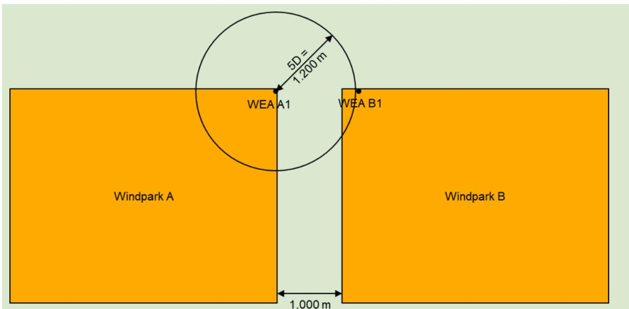
Illustration 6 Example schematic representation of a sequential commissioning of neighbouring OWPs according to the current regulation. Assumption: OWP A goes into operation before OWP B, both OWPs use a turbine type with a rotor diameter of 240 m
