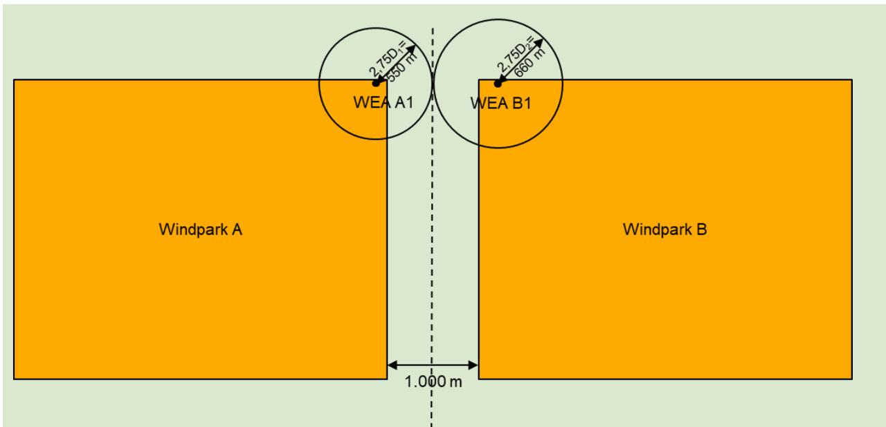
Figure 7 Supplement to the distance between wind turbines in neighbouring areas Variant 2: Assumption:  $D_1 = 200\text{m}$ ,  $D_2 = 240\text{m}$ , resulting distance between the turbines is 1,210m. This corresponds to  $6.1 \cdot D_1$  and  $5.0 \cdot D_2$ .
