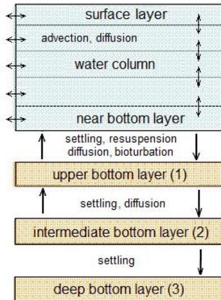
**Fig. A.1.** Vertical structure and radionuclide transfer processes in the compartment model POSEIDON-R.
