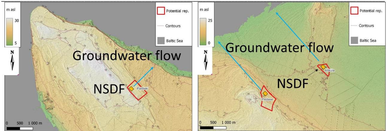
Fig. 3.2. Schematic directions of the groundwater flows (blue arrows) for different locations of the repository unit.
