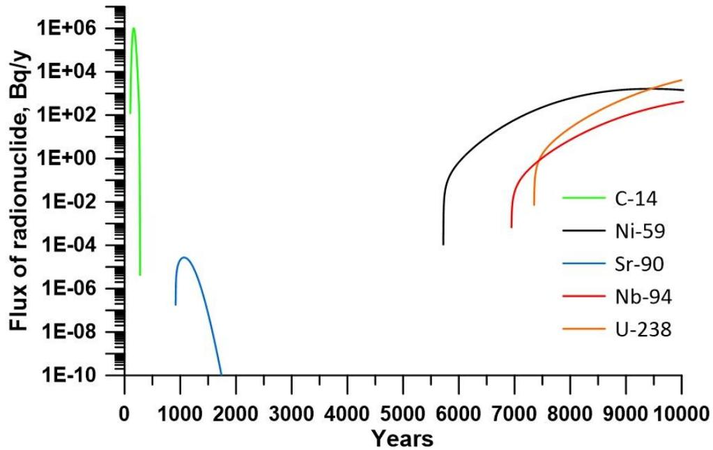
Fig. 3.3. Fluxes of radionuclides for the NSDF located at the PAL site used as a source term for the box 30 in the POSEIDON-R model.
