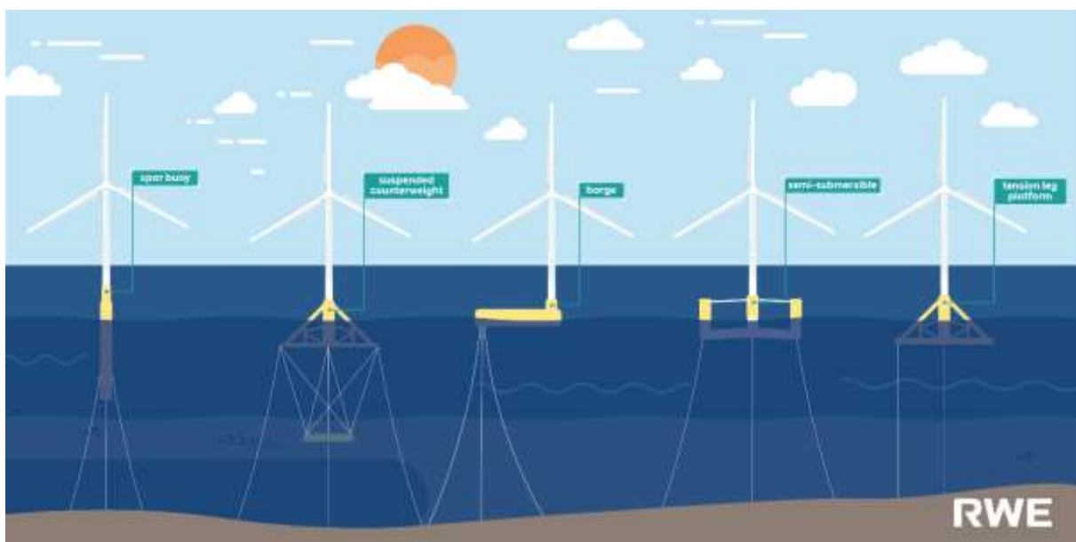
Figure 5. Different types of floating foundations.
