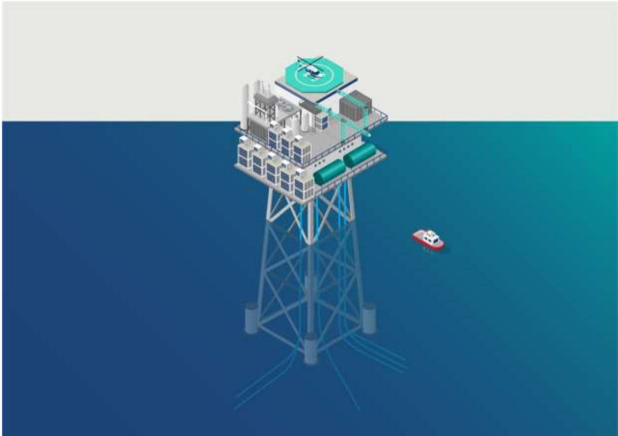
Figure 10. Illustration of substation on jacket foundation.
