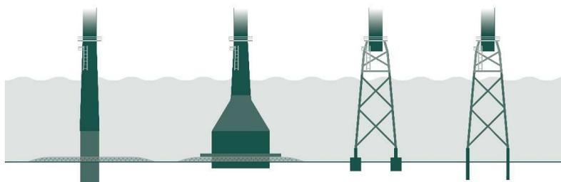
Figure 3. Principle sketch of bottom-fixed foundation alternatives. (From left: monopile foundations, gravity foundations, jacket foundations with suction buckets and jacket foundations with pin-piles). Source: LandInfra.
