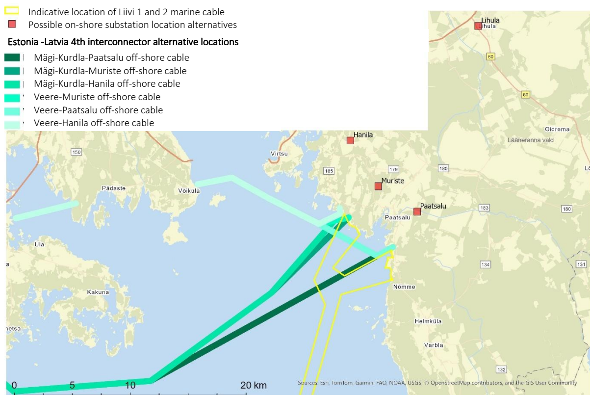
Figure 3.2. The proposed landfall site of the Liivi 1 and 2 offshore wind farm offshore export cable, and the alternative locations of the Estonia–Latvia 4th electricity interconnection submarine cable and the substation to be built in the Paatsalu area (according to the Estonia–Latvia 4th electricity interconnection map application data).
