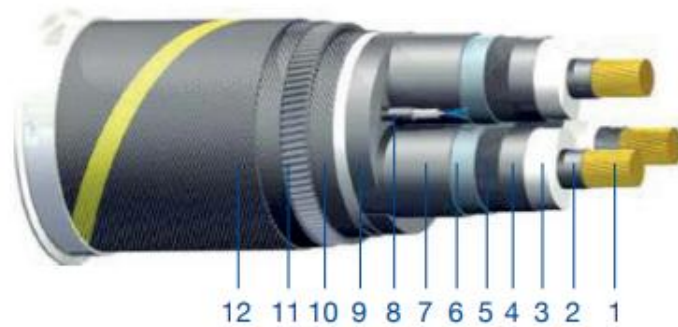
Figure 2.3.4.3. High voltage cable offshore cable up to 420 kV, (1) Conductor (Al or Cu), (2) Inner semi-conducting layer, (3) XLPE insulation, (4) Outer semi-conducting layer, (5) Swellable tape, (6) Lead sheath, (7) PE oversheath, (8) Fibre optic cable, (9) Filler profiles, (10) Bedding (PP), (11) Armouring, (12) Outer serving (PP). Source: NKT, (A)2X(F)K2YRAA
