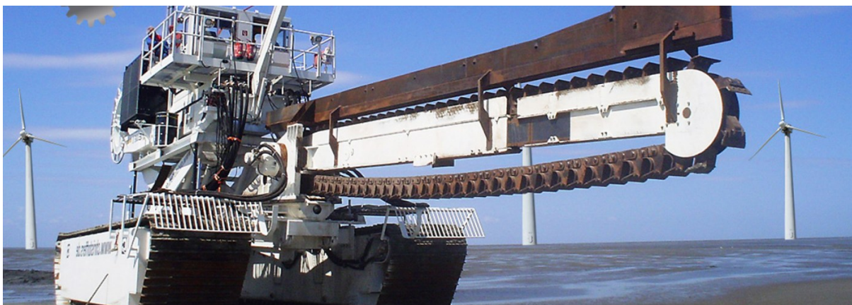
Figure 3.14 Equipment for burying cables in the seabed. Source: https://www.barthhollandrain.nl/page/161
