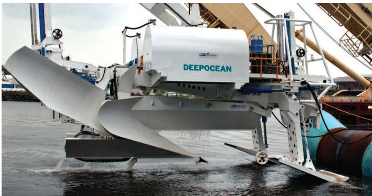
Figure 3.15 AMP500 advanced multi-pass plough. Source: https://www.subsea-rov.com/services-assets/trenchers-ploughs/item/74-amp500
