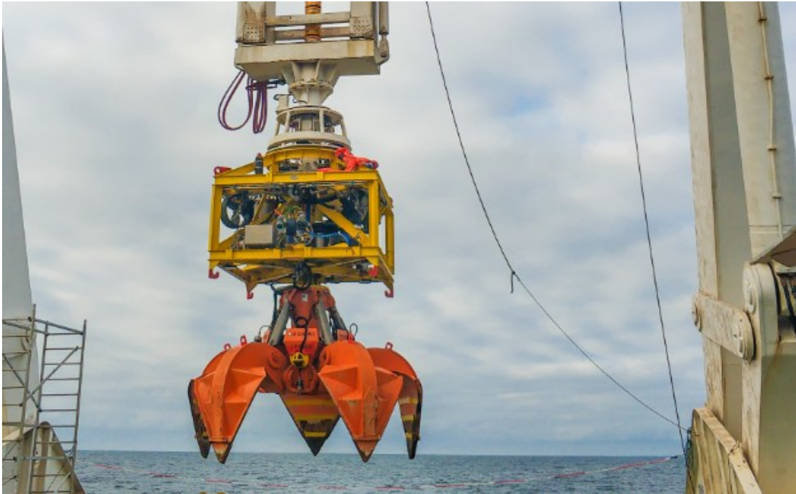
Figure 3.10 AssoGrapple II – a multi-purpose tool designed for seabed intervention (source:
