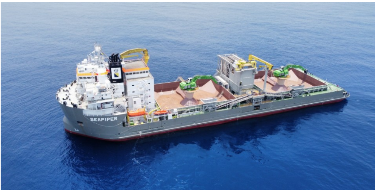
Figure 3.8 Example of a fallpipe vessel (source: https://www.portalmorski.pl/zegluga/53382-nowy-podsypkowiec-boskalisa )
