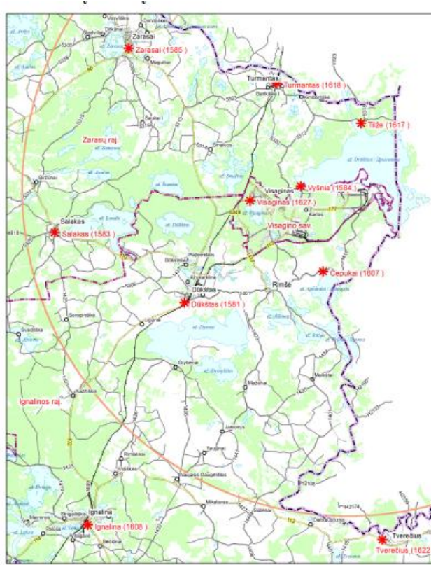
Figure 2.1-9 Layout of the Skylink system gamma detectors within the INPP 30 km zone
