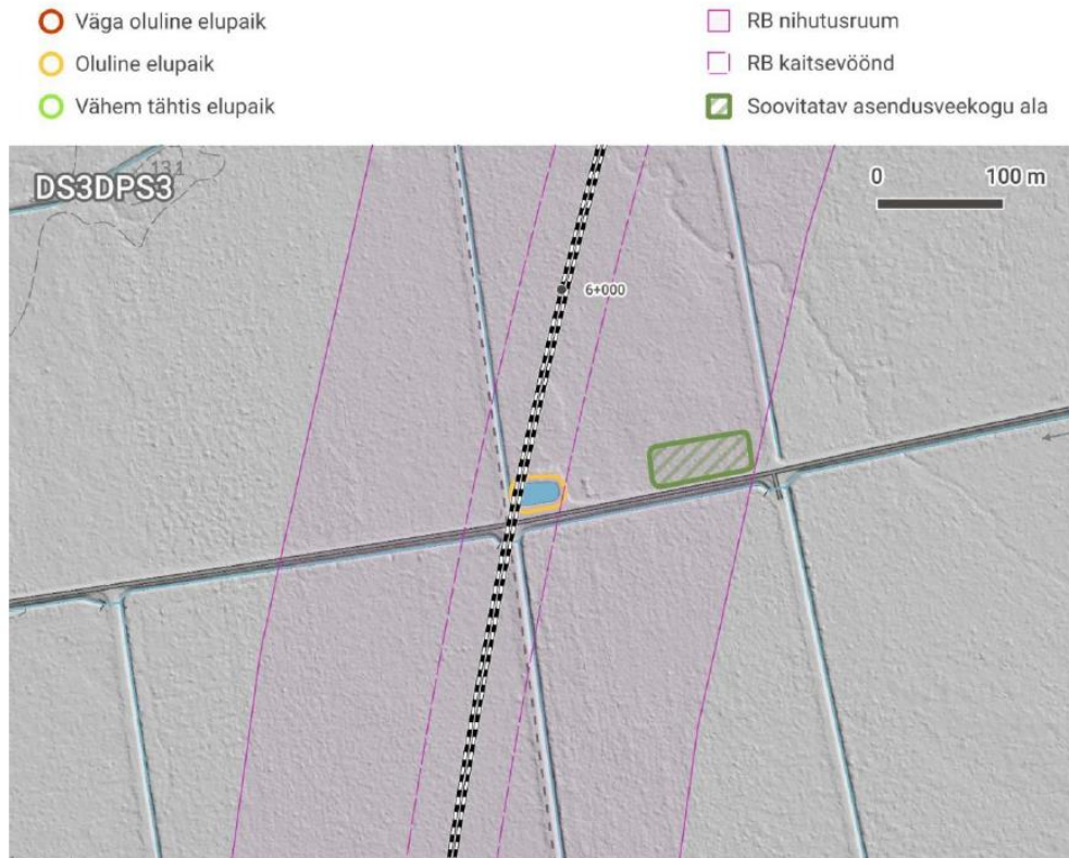
Figure 10-1. Location of the amphibian breeding water body in the railway corridor (kilometre 6+170) and recommended location of the replacement pond (source: OÜ Rewild, 2024. Amphibian habitats in Pärnu County on the RB DS3DPS3 section).
