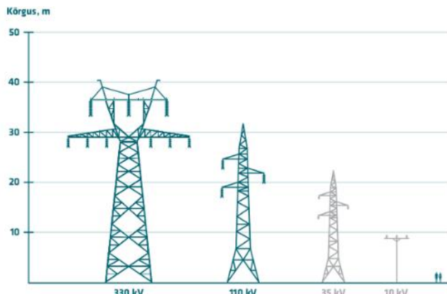
Figure 53. Pylons for overhead lines with different voltage classes. Source: Elering AS.
