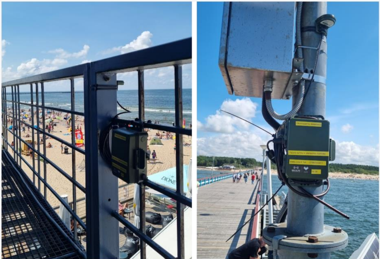
Fig. 5.4.66. Bat detectors installed on the Palanga lifeguard station (Palanga1) on the left and on the Palanga bridge (Palanga2) on the right.
