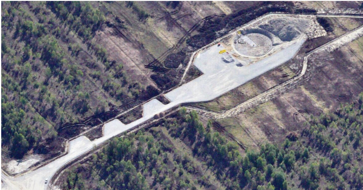
Figure 5. Possible wind turbine foundation area with assembly sites. Source: Land Board Kaldaerofoto – Tootsi/Sopi wind farm.
