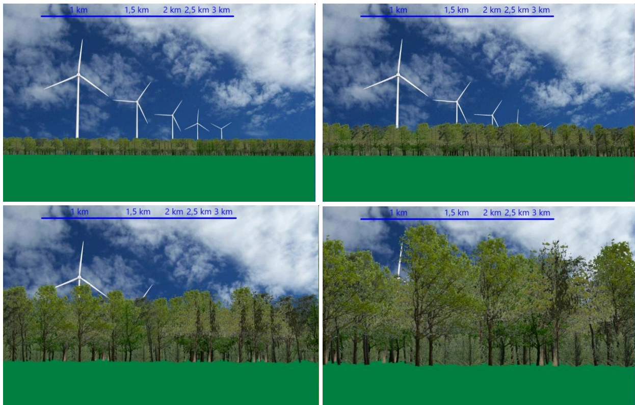
Figure 76. 270 m high wind turbines at distances of 1, 1.5, 2, 2.5 and 3 km, illustrated with a 20 m forest is located at distances of 500, 250, 100 and 50 m from the viewer.
